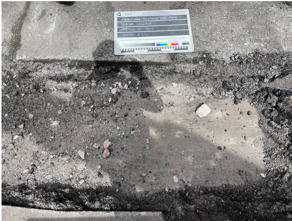
TS09 - Excavation to a depth of 0.30 m looking northwest - concrete encountered
