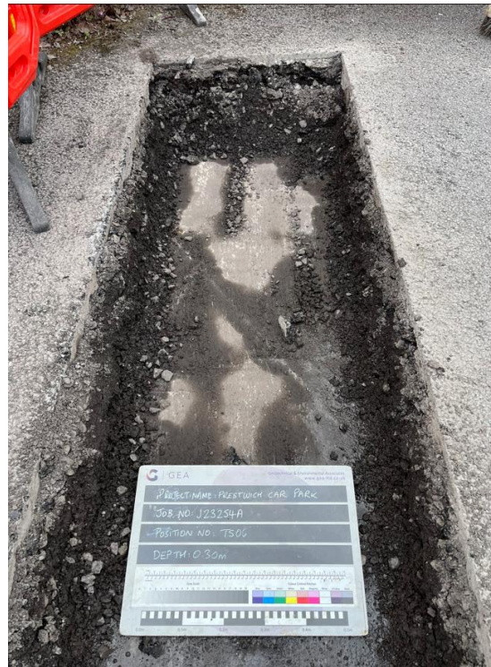
TS06 - Excavation to a depth of 0.30 m looking northwest - concrete encountered
