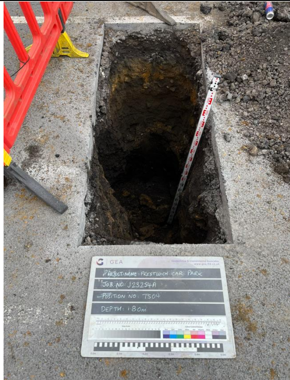
TS04 - Excavation to a depth of 1.80 m looking northwest - drainage pipe encountered
