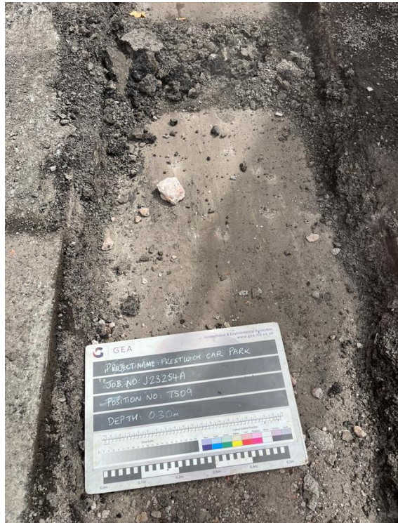
TS09 - Excavation to a depth of 0.30 m looking northeast - concrete encountered
