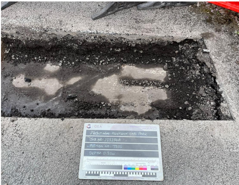
TS06 - Excavation to a depth of 0.30 m looking southwest - concrete encountered
