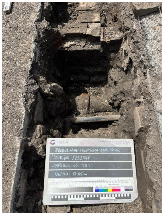
TS01 - Central part of the excavation to a depth of 0.85 m looking southwest containing drainage pipe and a black duct
