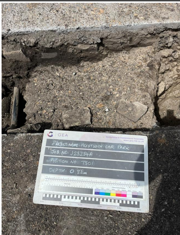
TS01 - Area of concrete within the central part of the excavation to a depth of 0.32 m looking northwest
