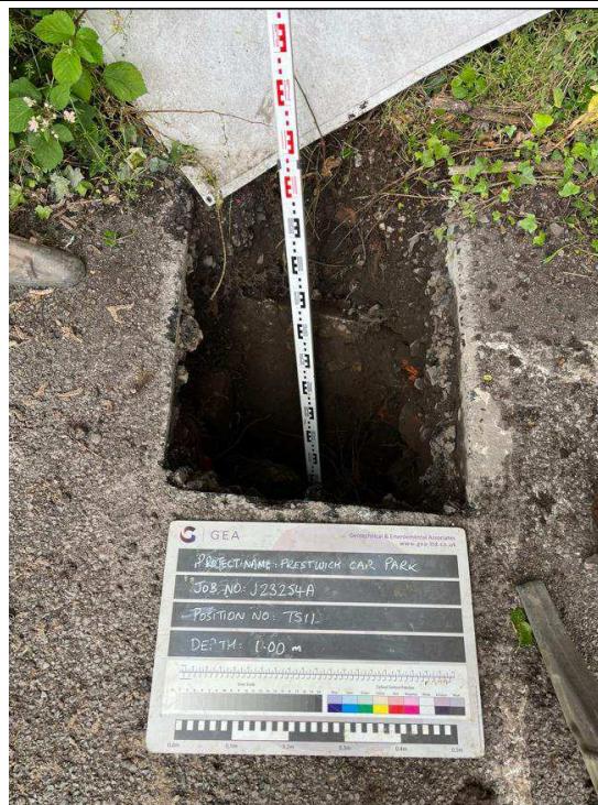
TS11 - Excavation to a depth of 1.00 m looking northeast - no services encountered
