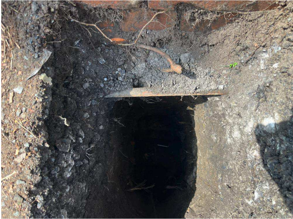
TP101 - Metal pipe encountered at a depth 0.16 m running parallel with the wall.
