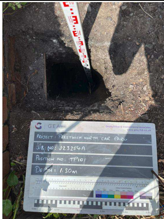
TP101 - Excavation to a depth of 1.30 m looking northwest
