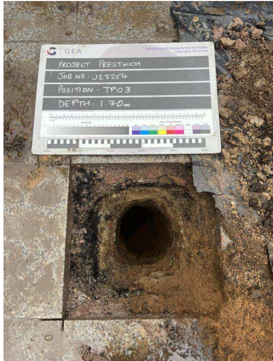
TP03 - Excavated to 1.70 m, looking east
