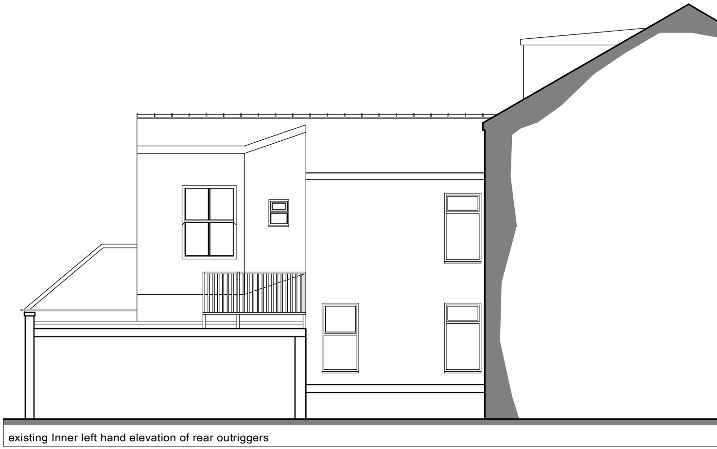
existing inner left hand elevation of rear outriggers
