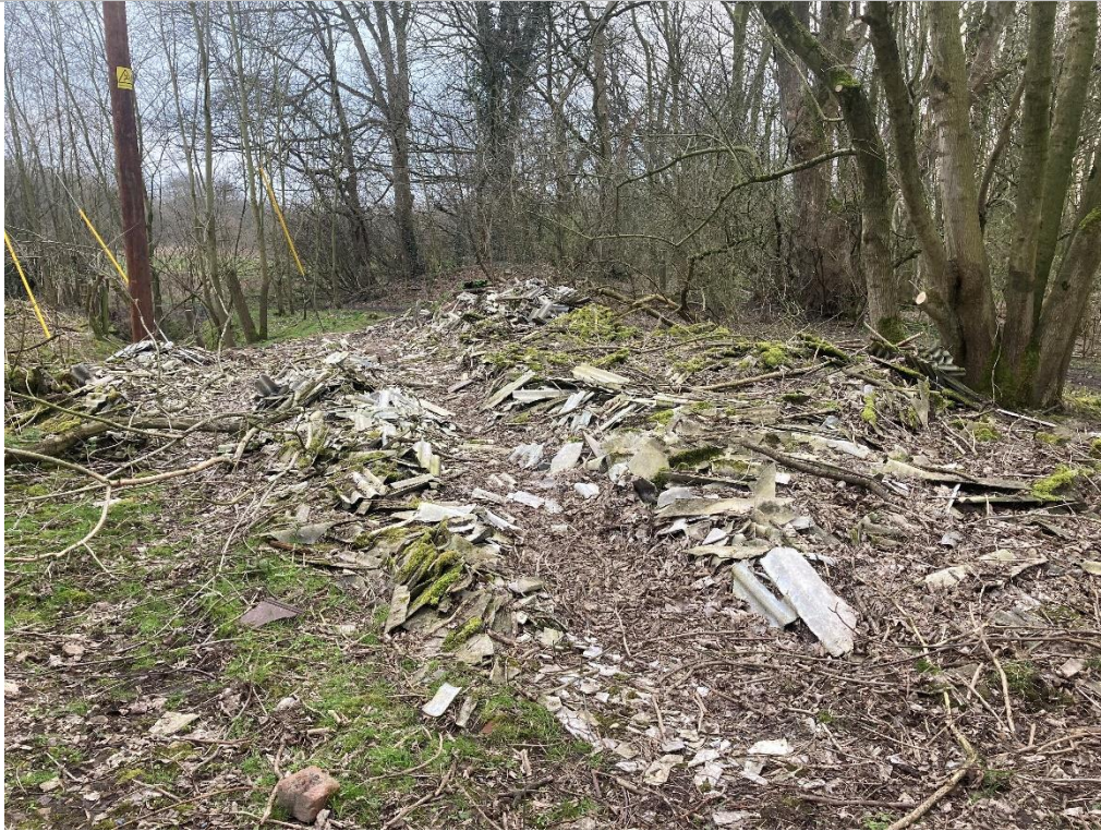
PLATE 9 ASBESTOS SHEET CEMENT SOUTH OF PEEL HALL
