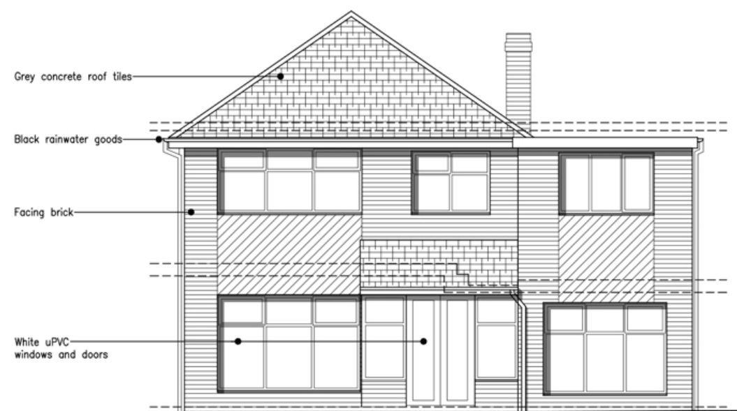
FRONT ELEVATION AS EXISTING
