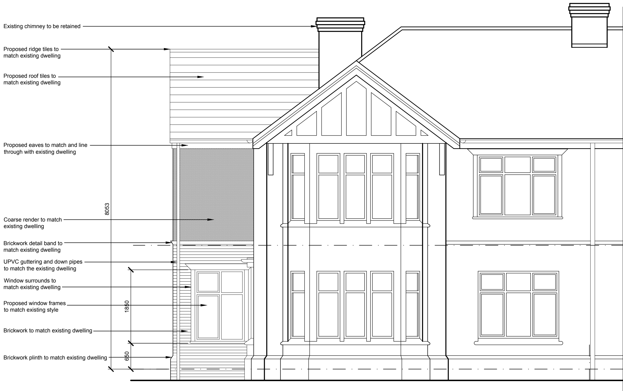
Front Elevation (West)
