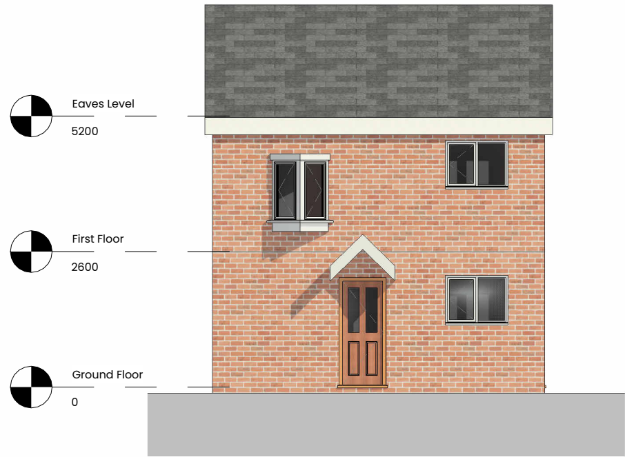
2 Existing Rear Elevation 1:100
