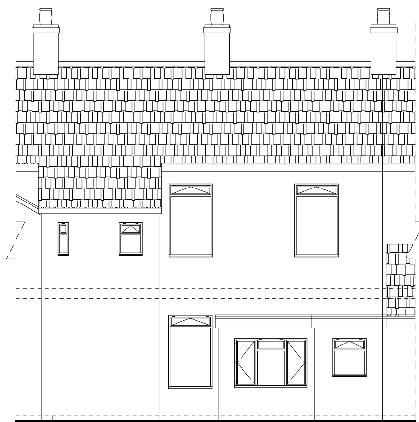
Existing rear elevation
