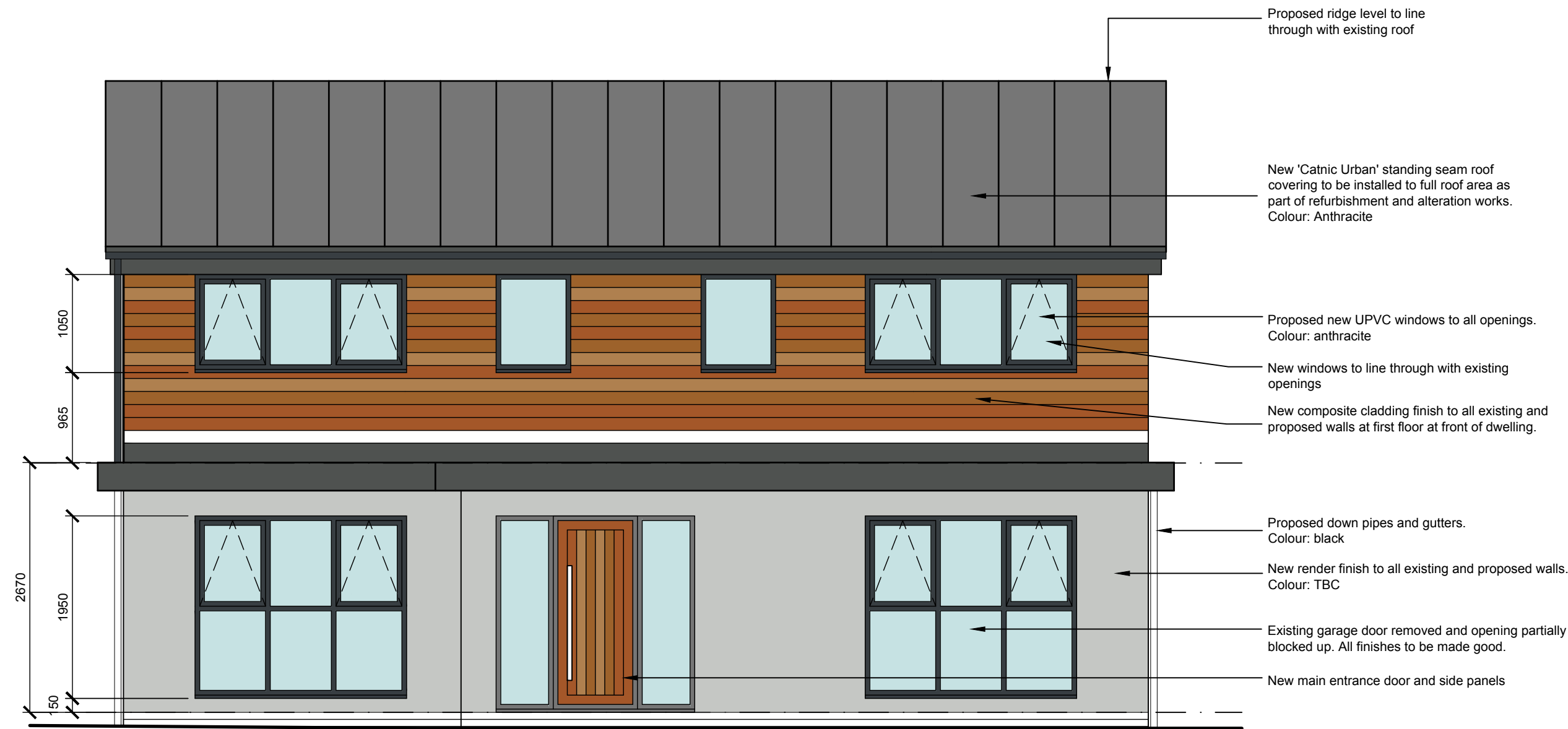
Front Elevation (Northwest)
