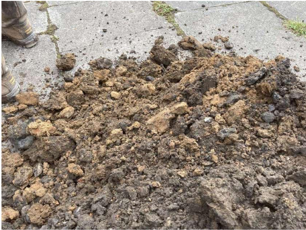
Plate 15 – TP2 >1.0mbgl arisings
