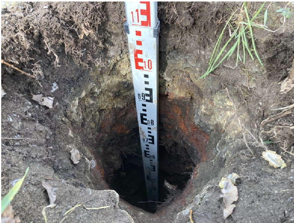
Plate 1 – Window Sampler 1 (WS1) hand pit to 1.2m below ground level (bgl)
