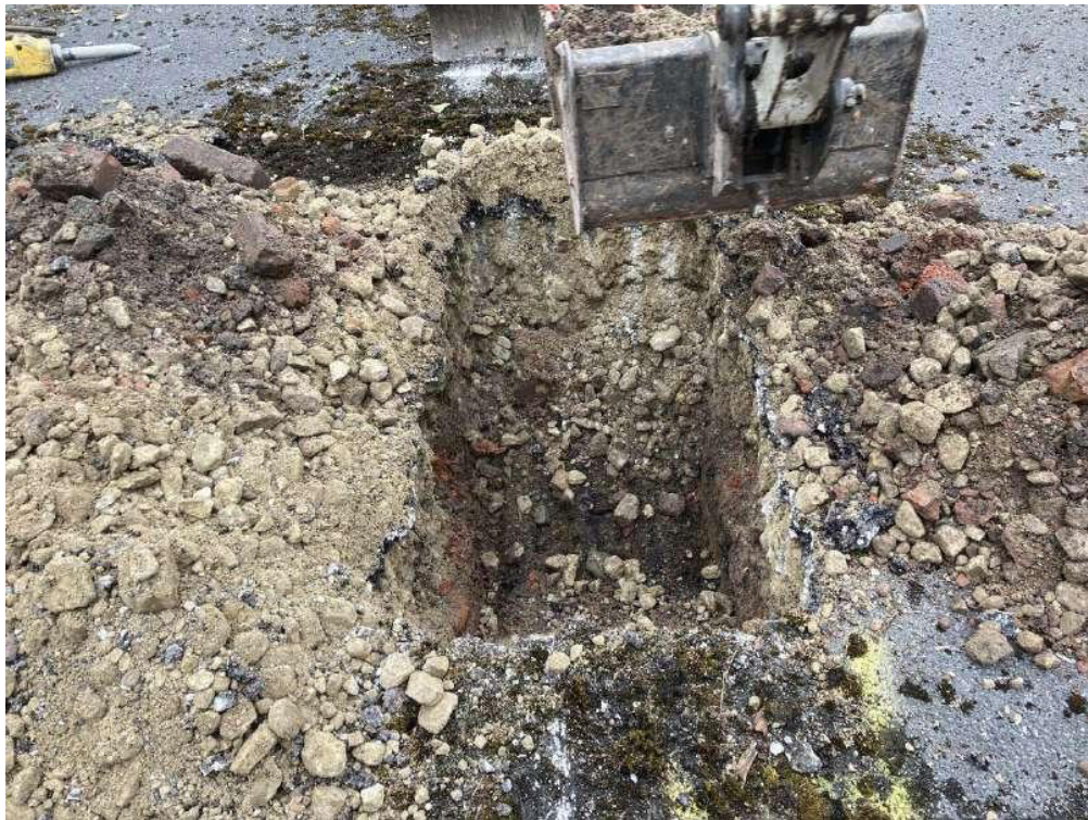
Plate 12 – TP4 gl to approximately 0.4mbgl with arisings
