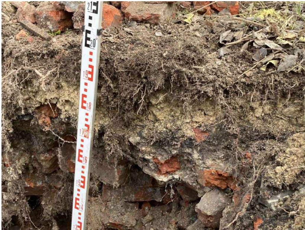
Plate 1 – Trial pit 1 (TP1) ground level to 0.5mbgl showing topsoil overlying sandstone gravel and cobbles
