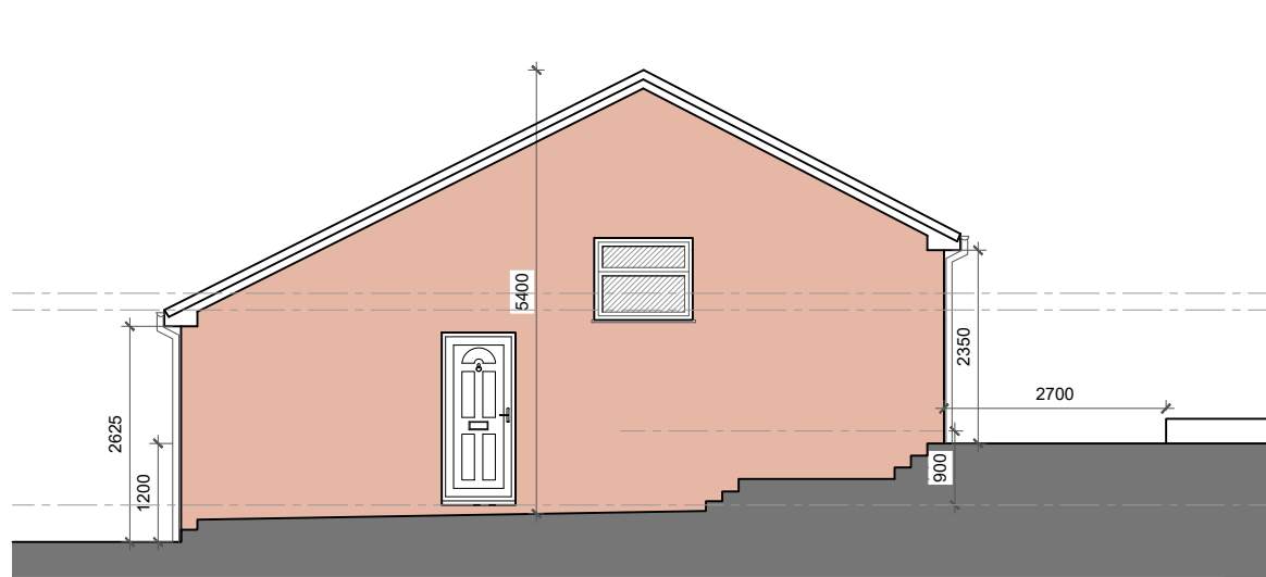
West Elevation 1:100 Existing
