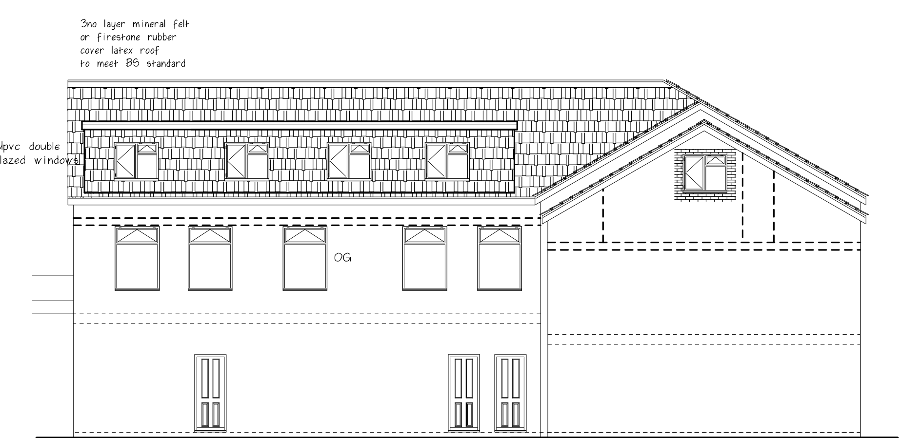
Proposed side elevation (Back Topping St)
