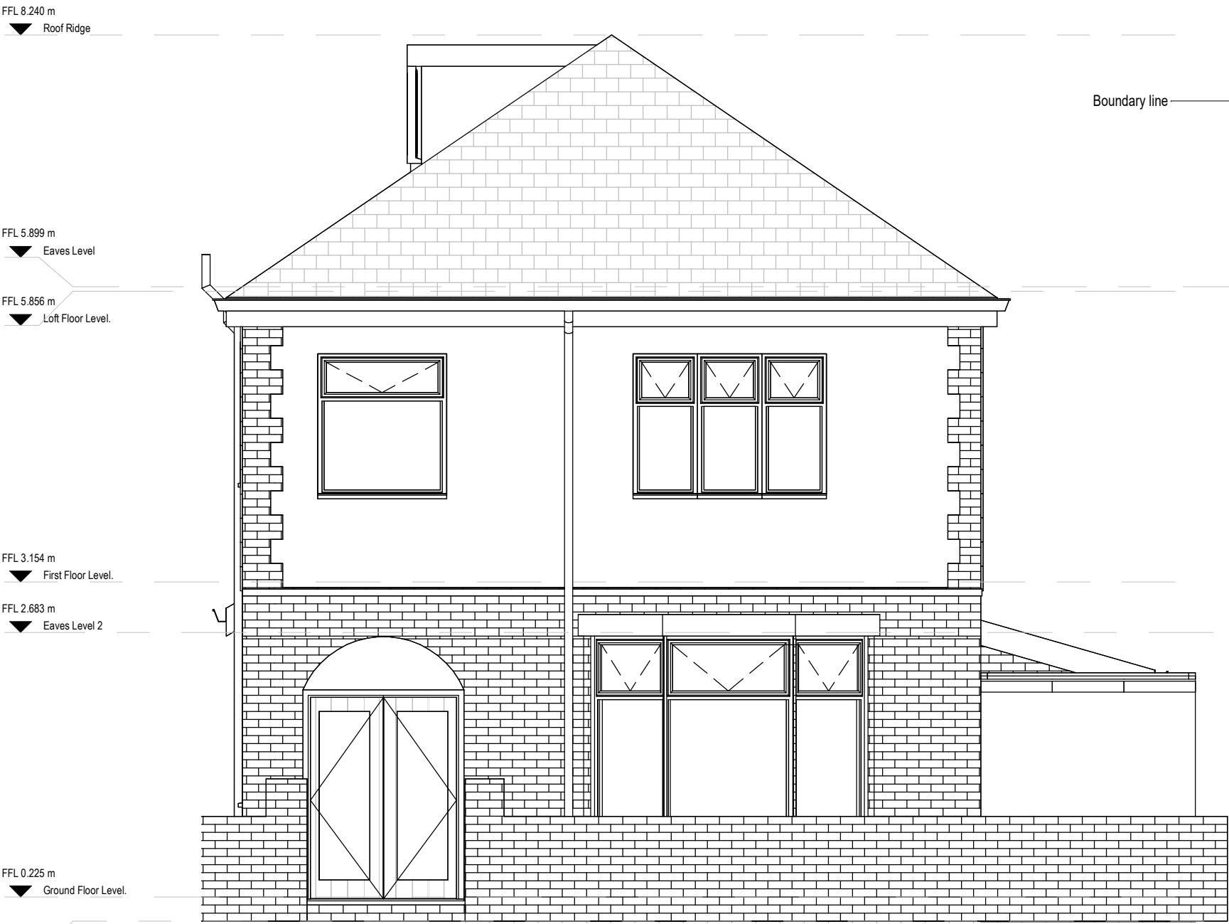
Existing Front Elevation 1 : 50
