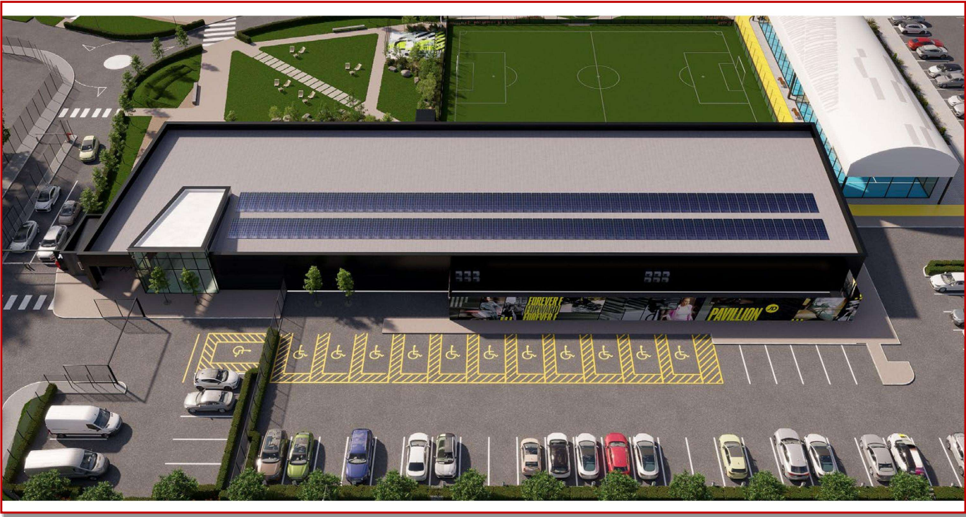
Figure 3 - Indicative PV Roof Layout
