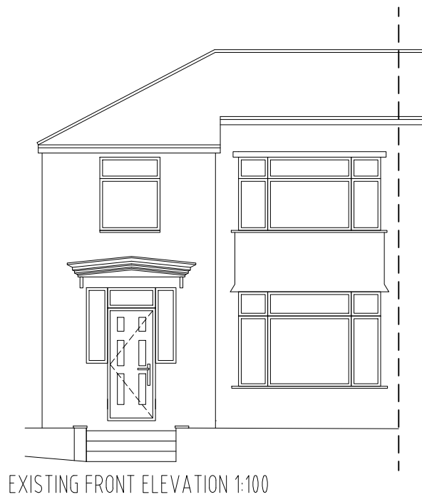
EXISTING FRONT ELEVATION 1:100
