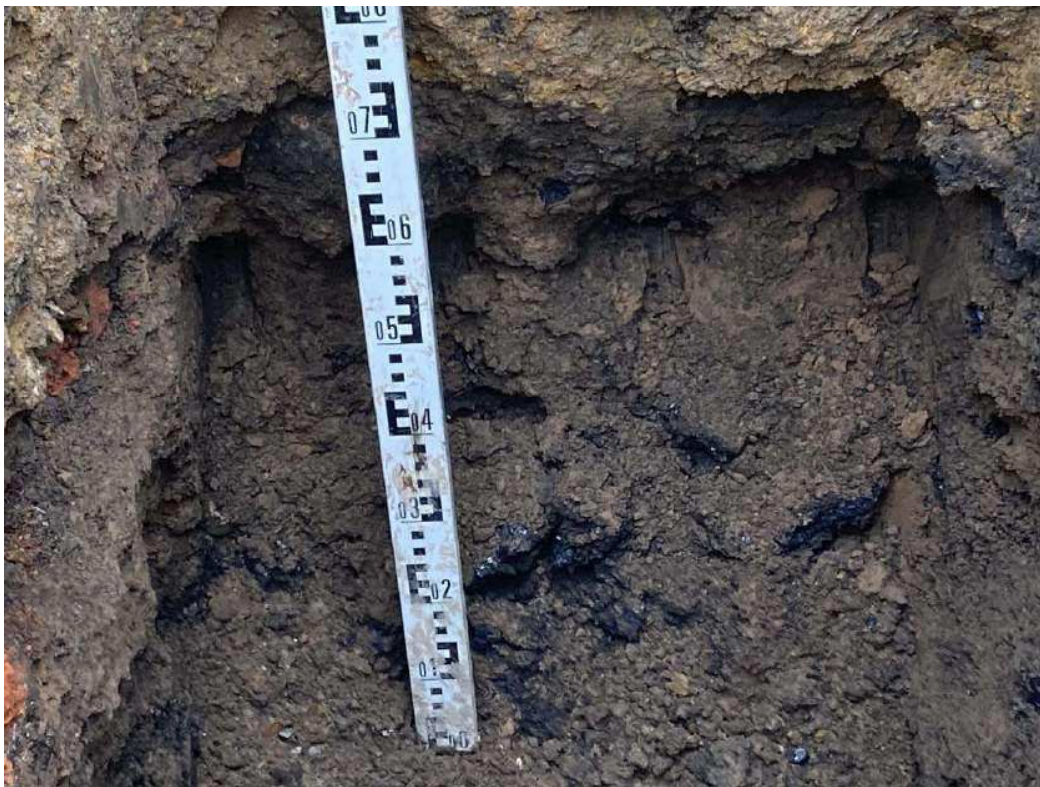
Plate 17 – TP4 natural ground with coal cobbles
