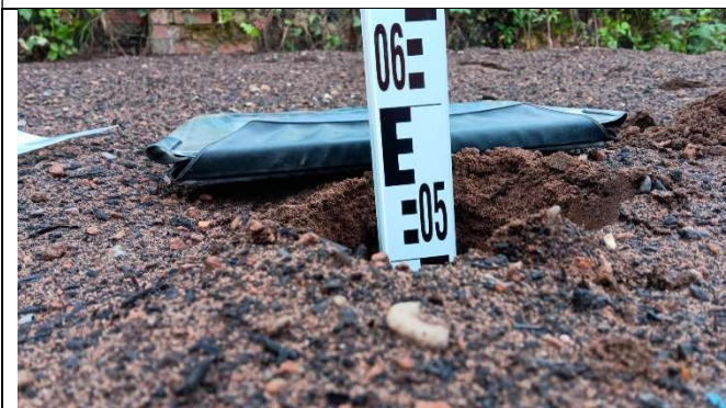
Depth measurement of pit 2 ( circa 570mm soil cover over membrane).
