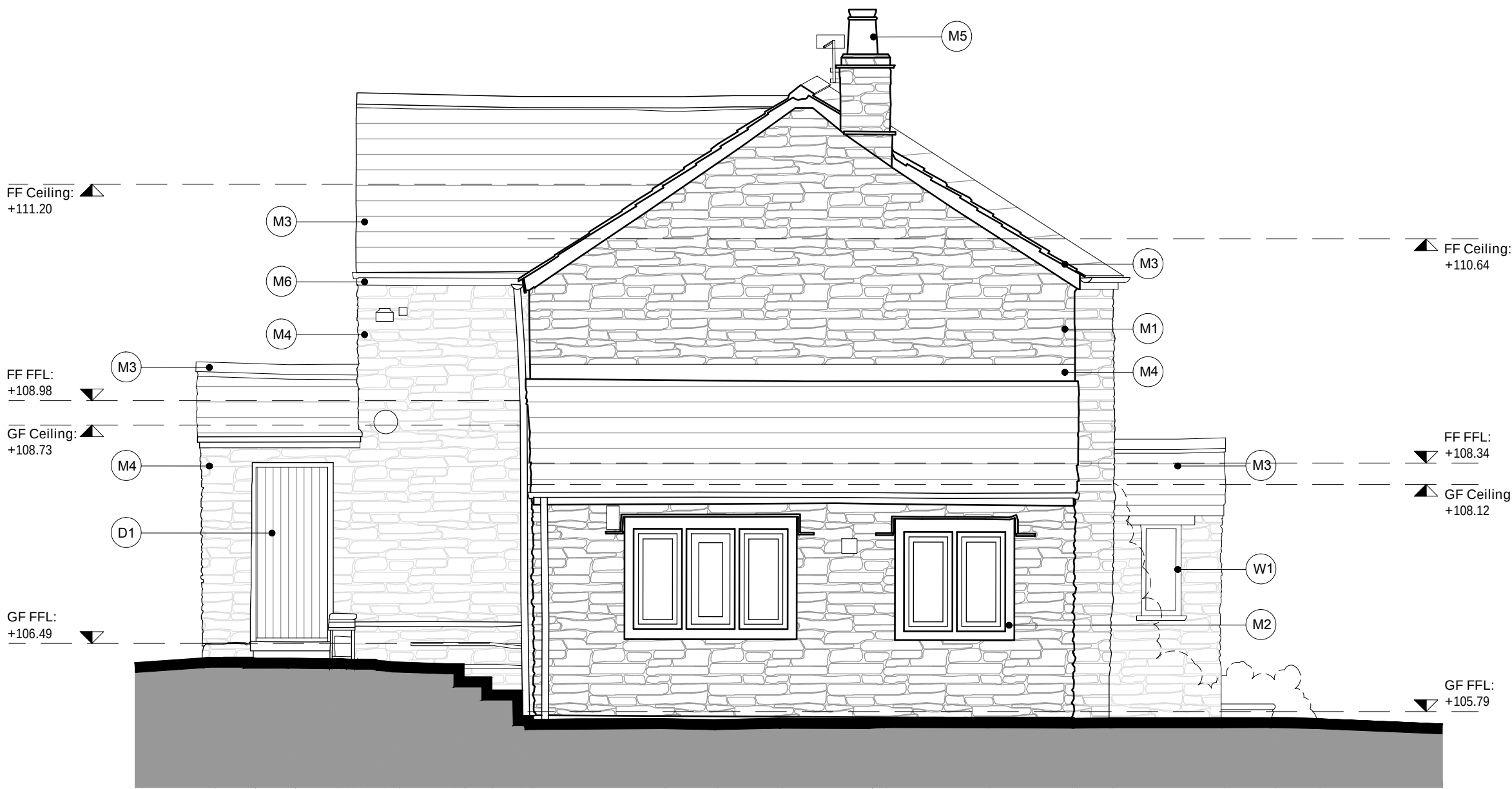
West Elevation as 'Existing' Scale 1:50
