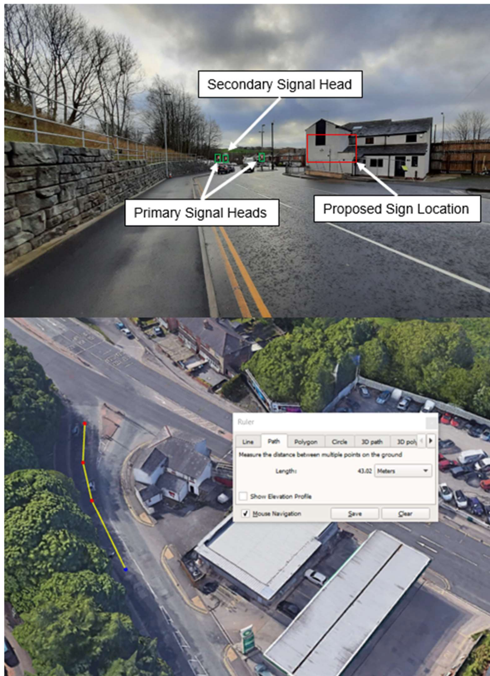
Figure 3.1 – South-eastbound Approach along B6221 Wash Lane at 43m SSD from Stop Line
