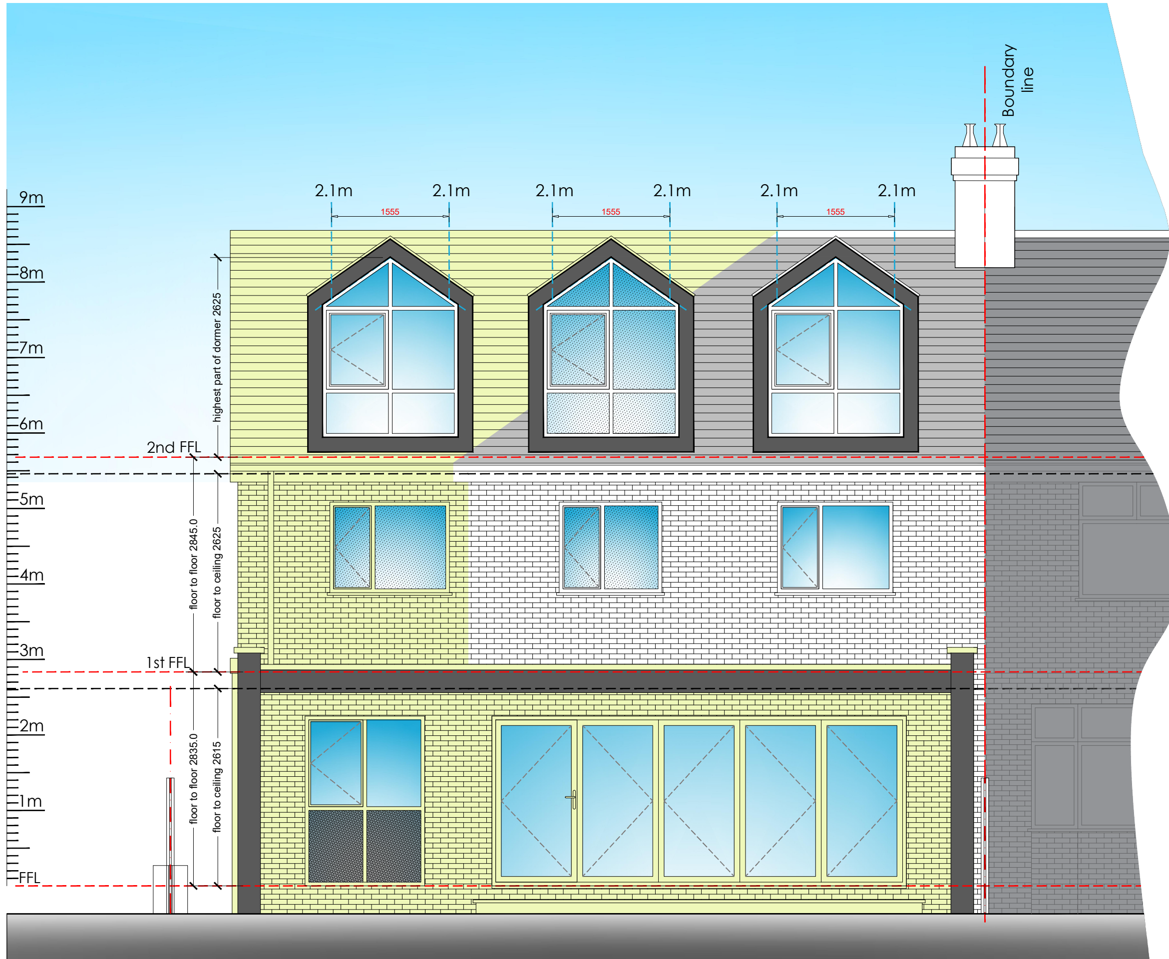
rear elevation - as proposed scale 1:50 at A1
