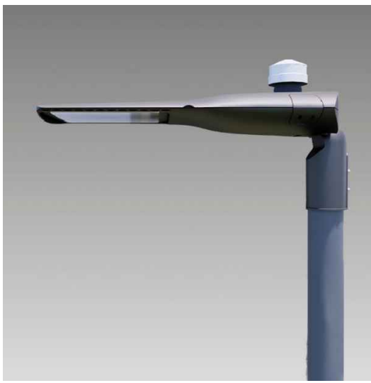
Steon : Condor Midi 150W LED Luminous Efficacy: 116lm/W Finish : Grey Powder Coated Aluminium Colour Temperature: 4000K Asymmetric 150° beam angle
