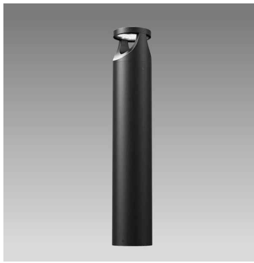
Steon : Monarch 14W LED Bollard Luminous Efficacy: 85lm/W Finish: Black Powder Coated Aluminium Colour Temperature: 4000K Dims Dia165mm xH900mm
