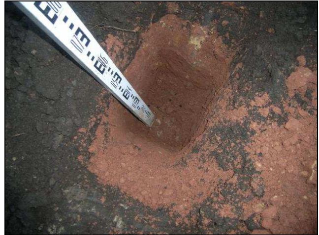
Photographs 1 and 2: Examples of validation photographs demonstrating validation hole location and soils forming inert cover.
