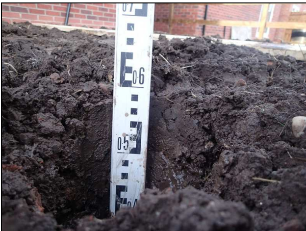
Photographs 3 and 4: Examples of validation photographs demonstrating inert cover depth and geotextile.
