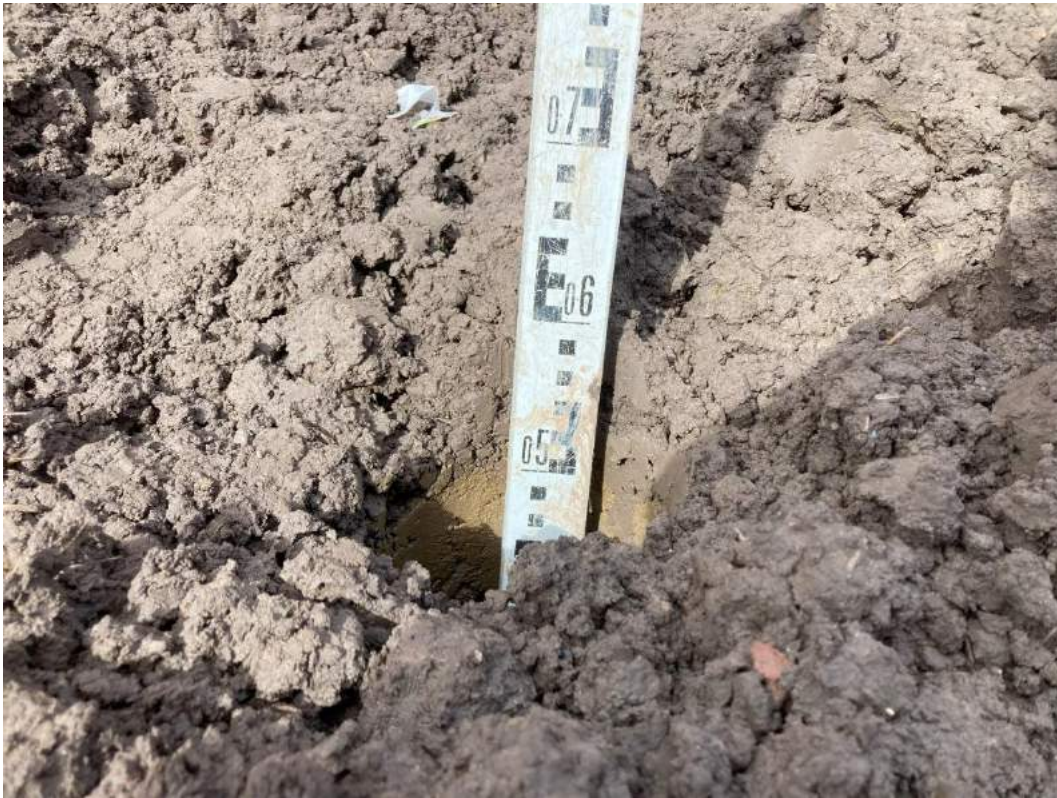
Plate 23 – Plot 5 front garden cover system GL to 0.60mbgl with 0.15m of topsoil.
