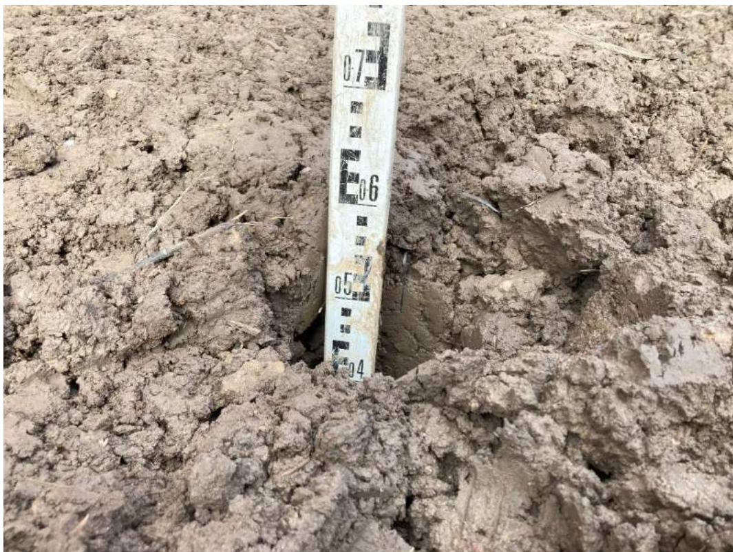
Plate 18 – Plot 4 front garden cover system GL to 0.60mbgl with 0.15m of topsoil.
