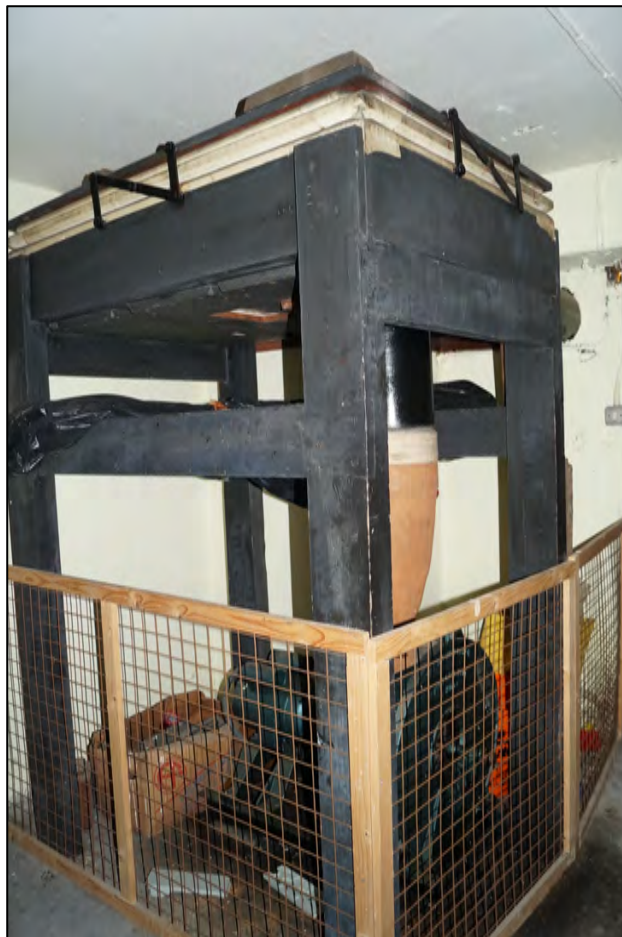
Plate 11. The pump mechanism for the organ.
