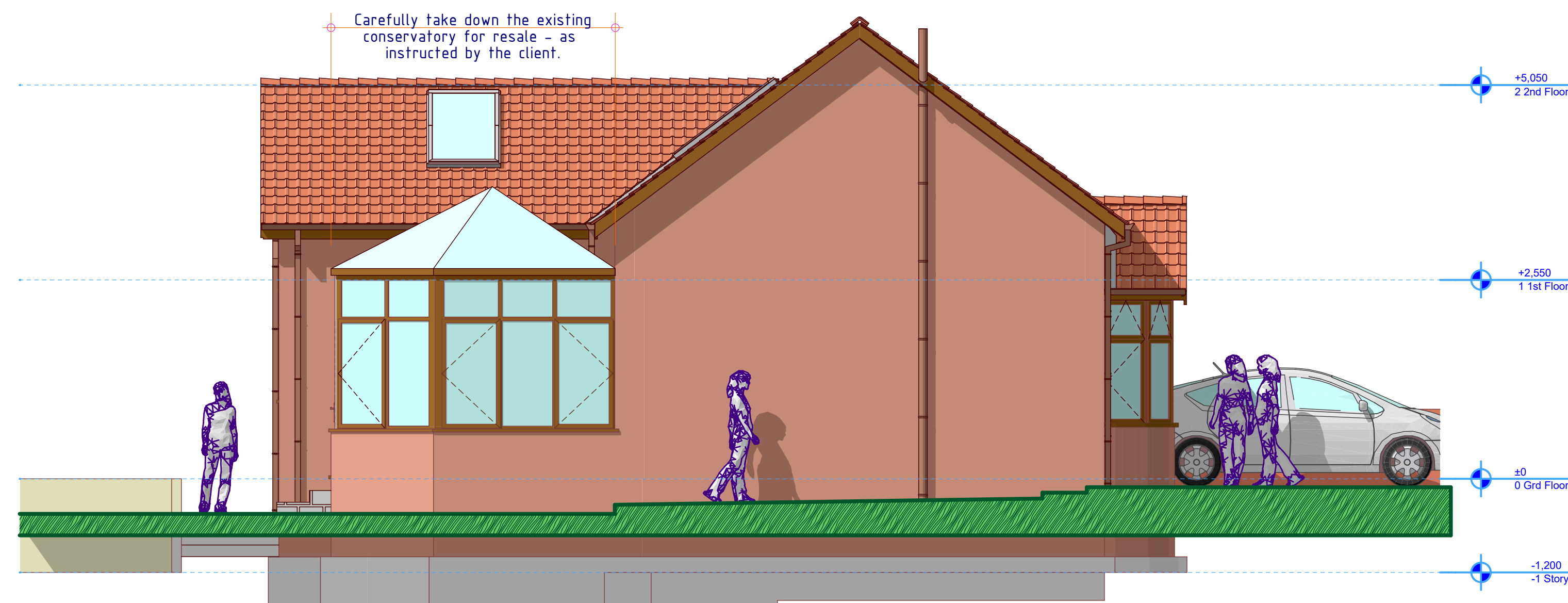
2 Existing Side Elevation 1:50
