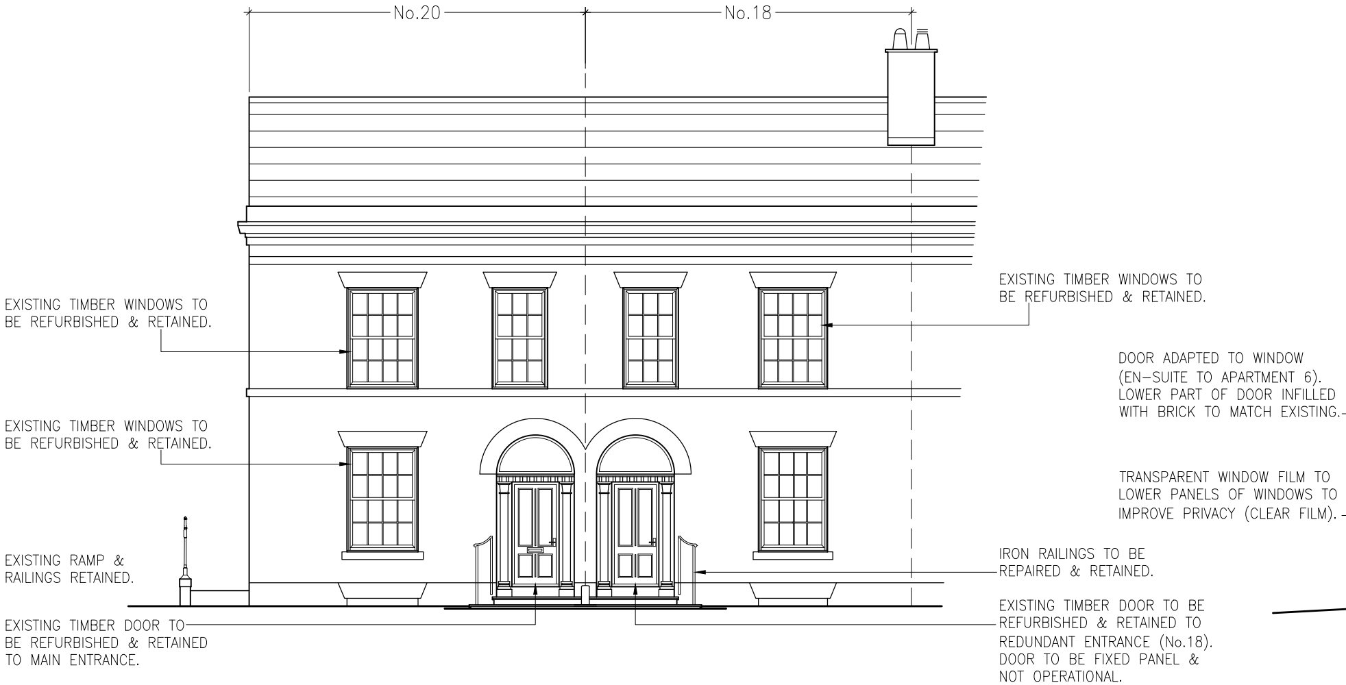
PROPOSED FRONT/SOUTH ELEVATION (1:100)
