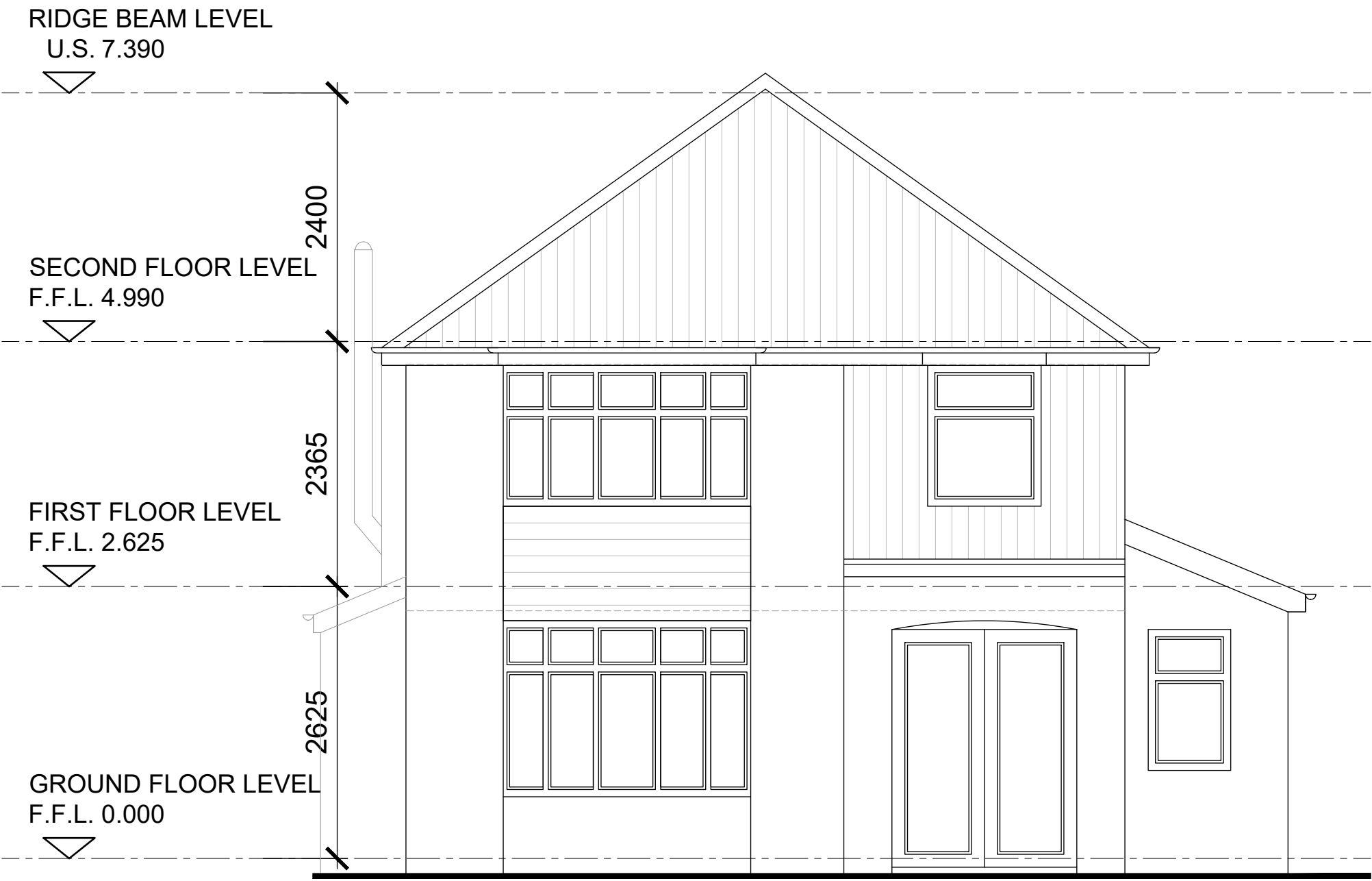
EXISTING FRONT ELEVATION
