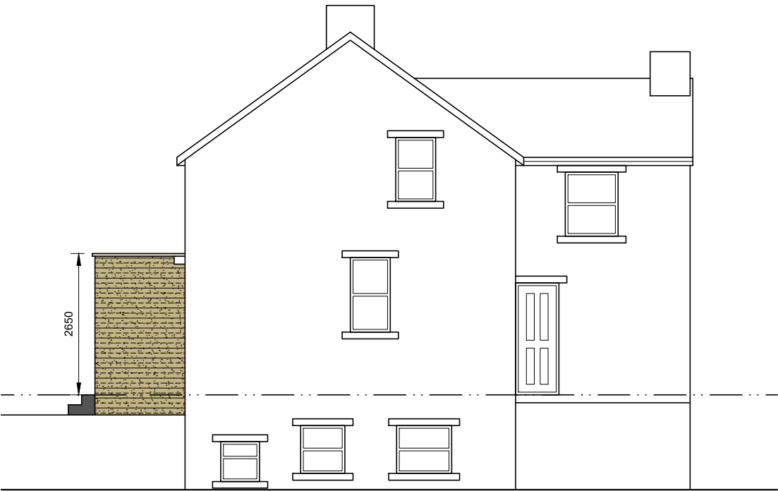
East Facing Side Elevation
