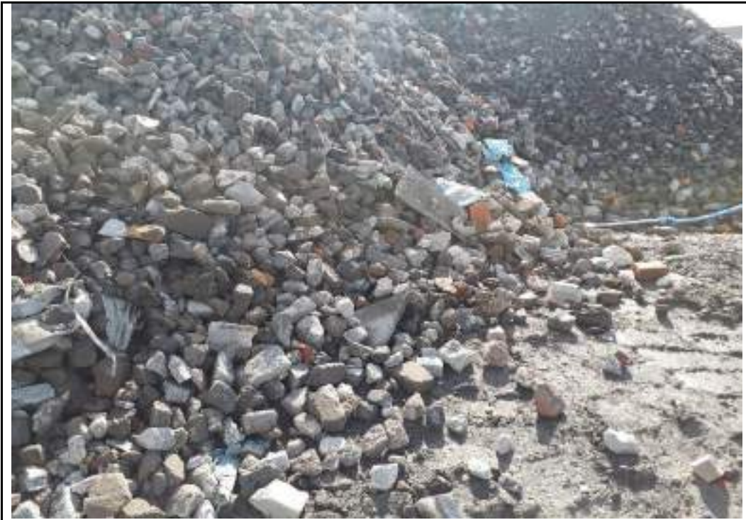
Photograph 113: Existence of deleterious material in stockpile of crushed material from oversize of the screener in eastern part of the site. VHE to confirm classification of coarse graded material
