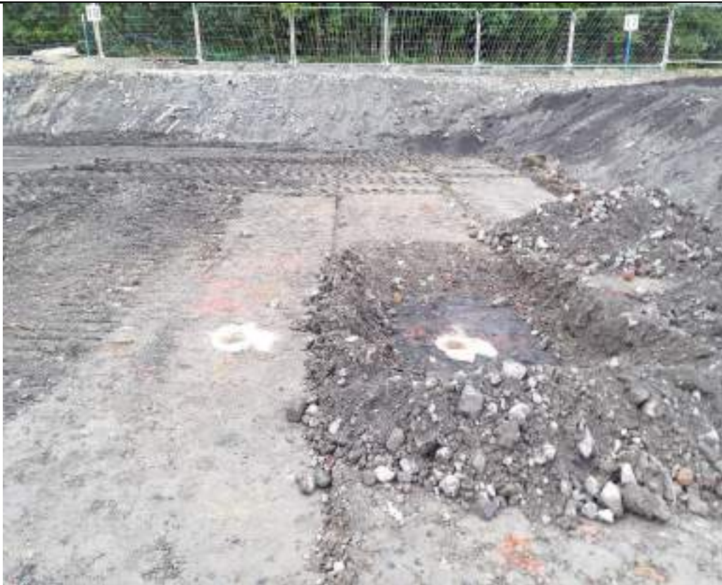
Photograph 26: Locations of SRD tests on fill material in southwestern part of the site.
