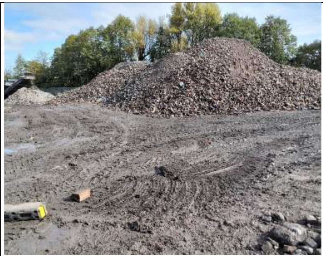
Photograph 10: Overview of stockpile of crushed material from oversize off screener.
