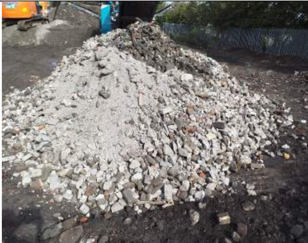
Photograph 8: Oversize material off screener after crushing by crusher in northeast of the site.
