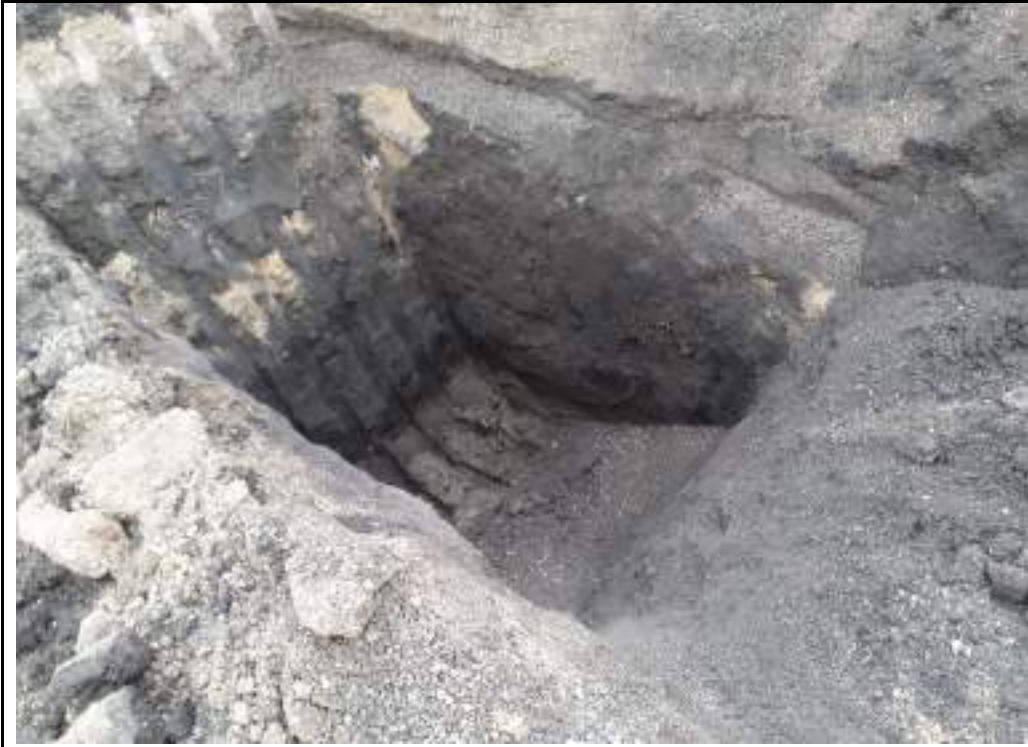
Photograph 23: Trial pit in location of organic Made Ground deposit in northeastern boundary of the site.
