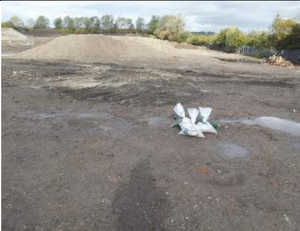
Photograph 22: Samples and backfilled trial pit in eastern part of the site.
