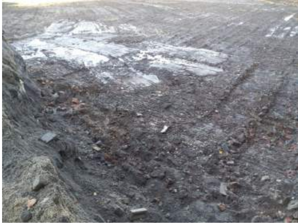
Photograph 5: Glacial Till formation in excavation in eastern part of the site.
