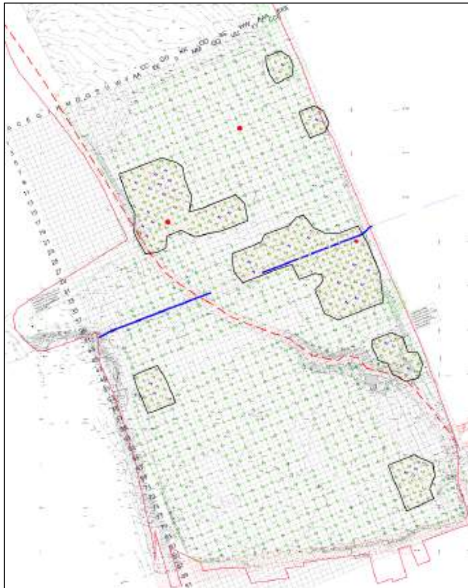
Figure 8: Extract of the completed drill and grout grid with areas requiring secondary holes outlined and highlighted in orange.
