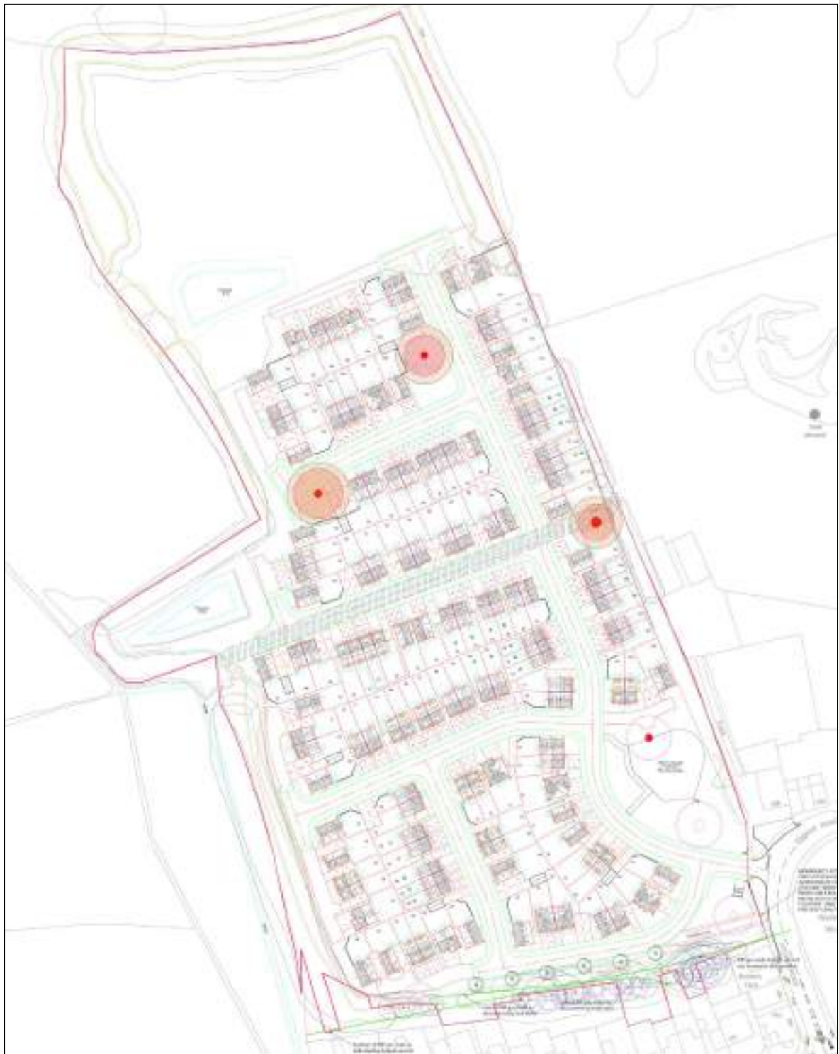
Figure 1: Extract of the proposed development plan rev AG – the layout also illustrates the three previously unrecorded mine entries in the north and eastern site sections (noted with a red dot and shading)
