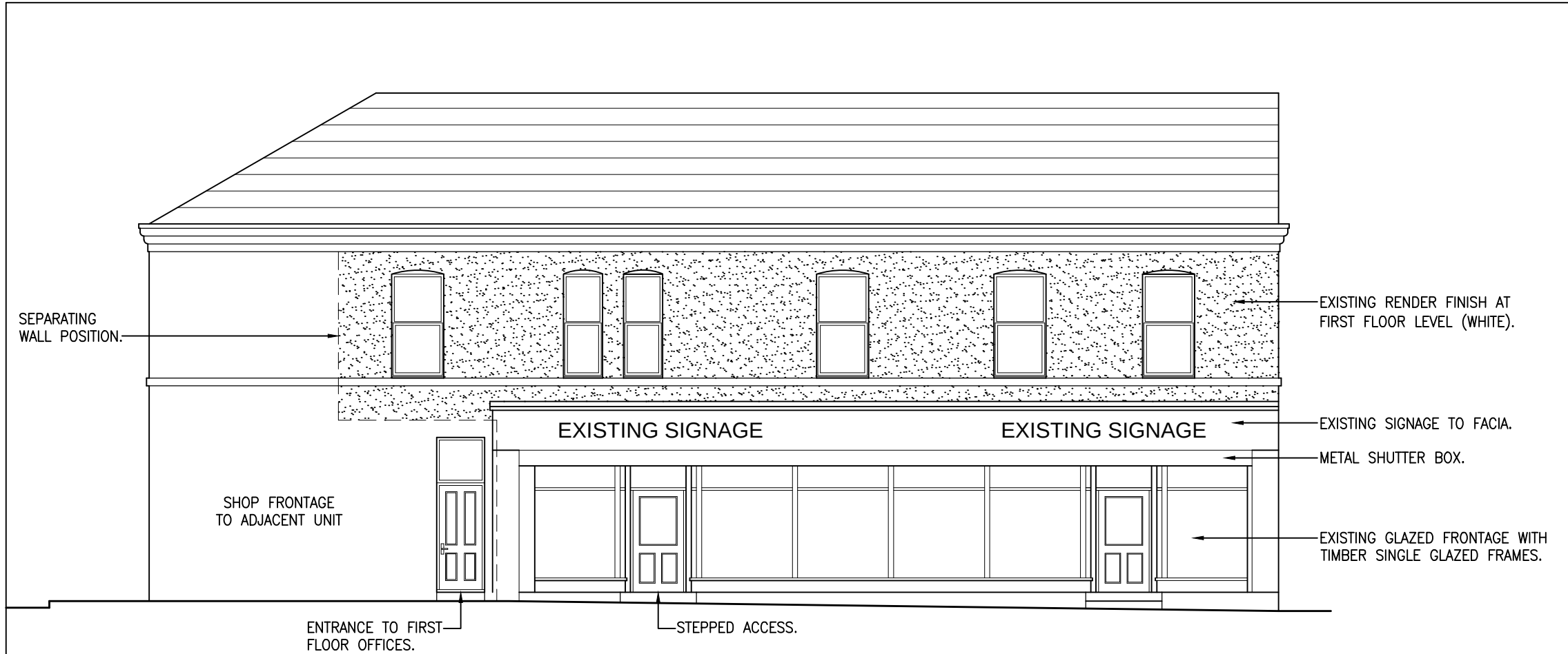
EXISTING FRONT ELEVATION (1:100)
