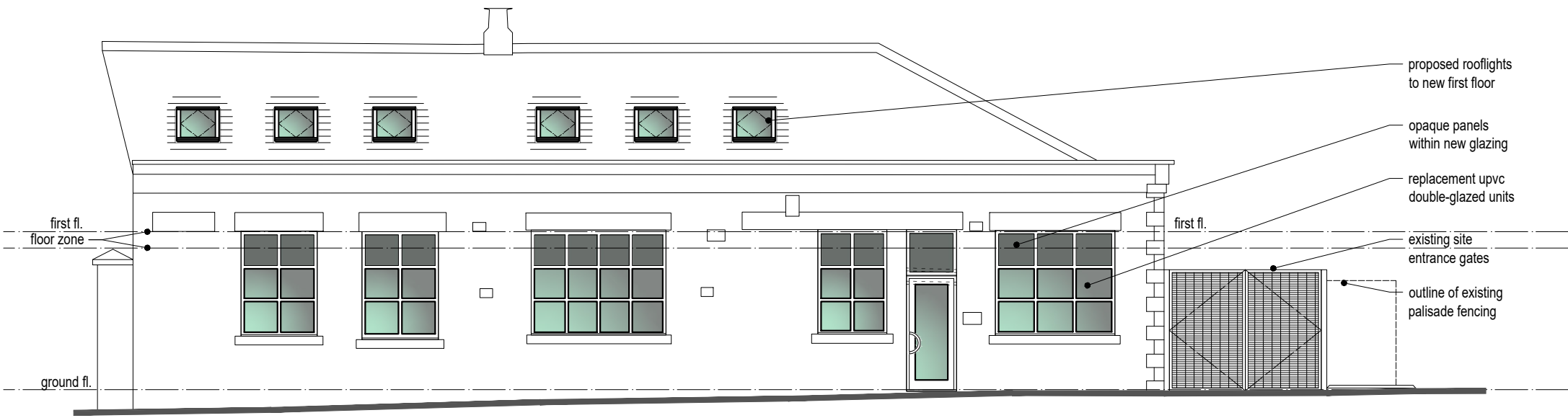
FRONT (SOUTH-EAST) ELEVATION
