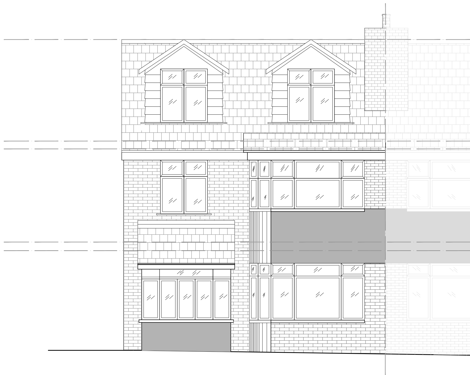
1 PROPOSED FRONT ELEVATION SCALE: 1/50
