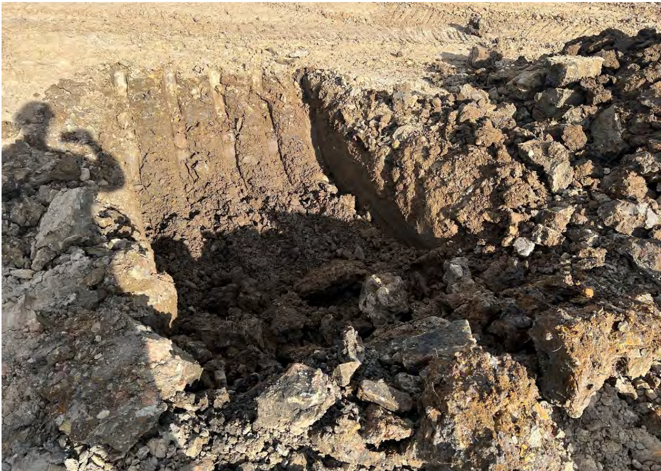
Photograph 30 – No evidence of organic material in pit to west.
