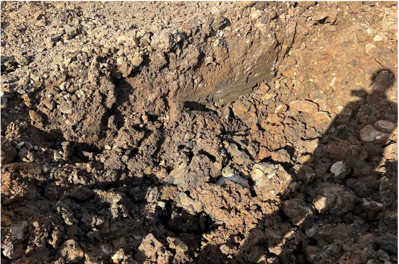
Photograph 31 – Trial pit to centre with limited silt detected.
