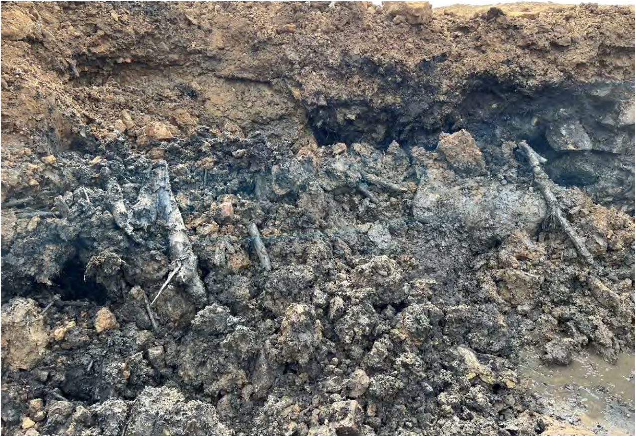
Photograph 29 – Deeper Made Ground with organic properties at the northern area of site – silt band thins out southwards.
