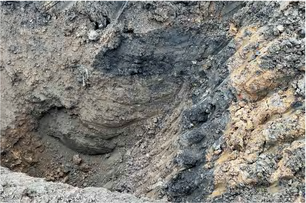
Photograph 25 – Band of silt beneath reworked clay at centre of site.
