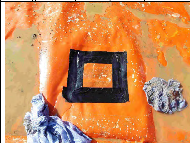
Plot 15: Patch repaired with double sided tape and single sided tape
