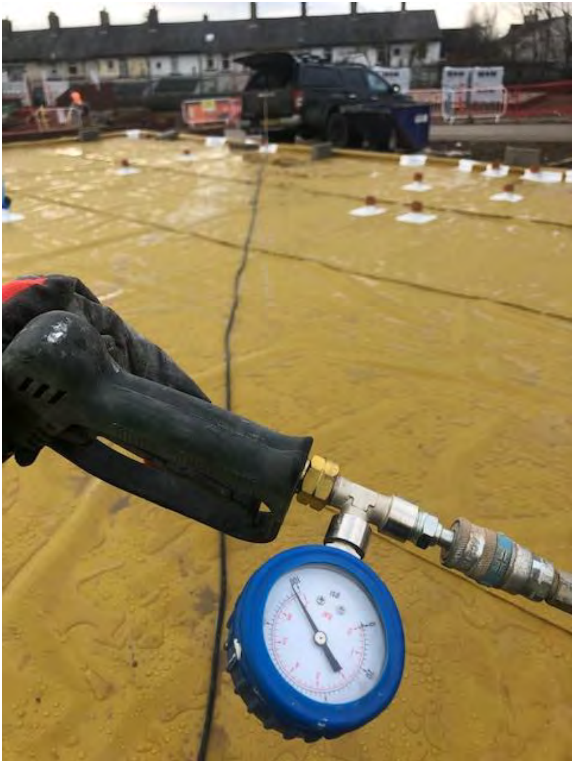
Barratt Bury Photograph 2: Air Lance Pressure Evidence:
