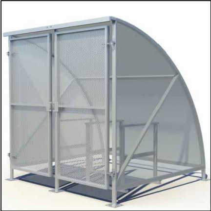
GALVANISED STEEL FRAMED CYCLE STORAGE SHELTER, FOR 10 CYCLES, 3260mm LONG x 2600mm WIDE x 2200mm HIGH, GATED FRAMES TO RECEIVE PERFORATED INFILL PANELS. PROVIDE 5no SHEFFIELD STANDS, FIXED TO TO HARD STANDING.
