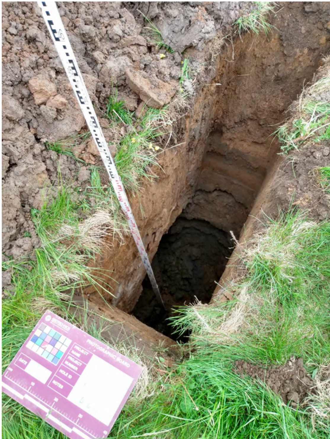
Machine-dug Trial Pit TP04 (2)
