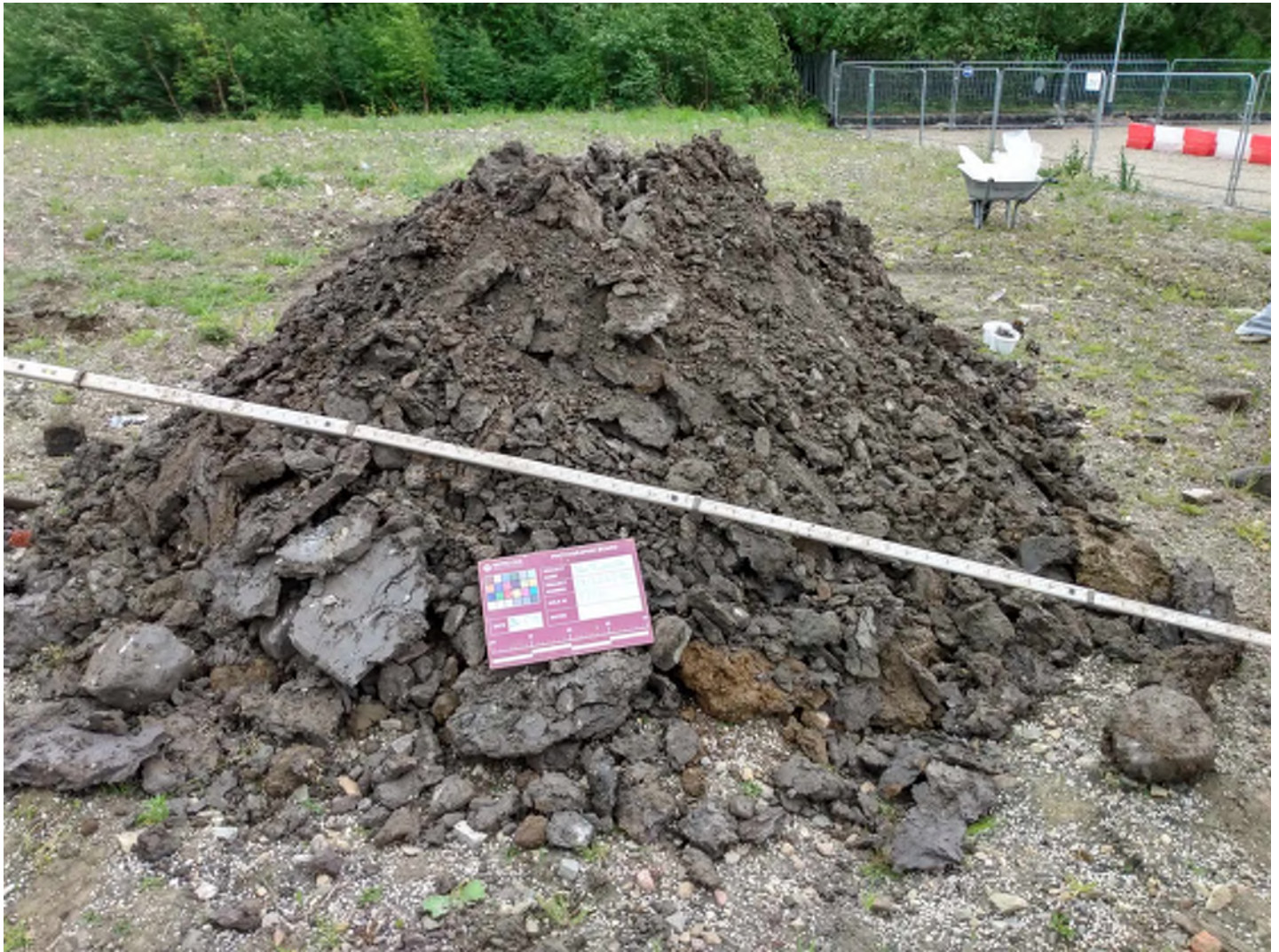
Machine-dug Trial Pit TP01 (5) Arisings
