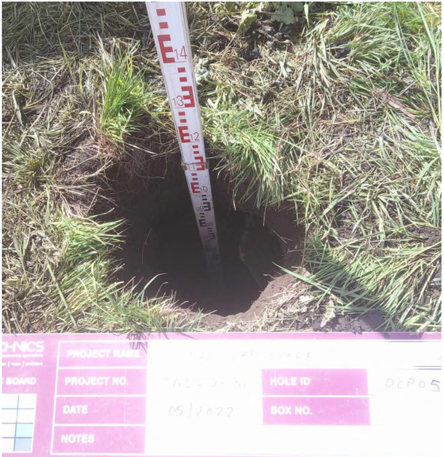
Hand-dug Trial Pit DCP05
