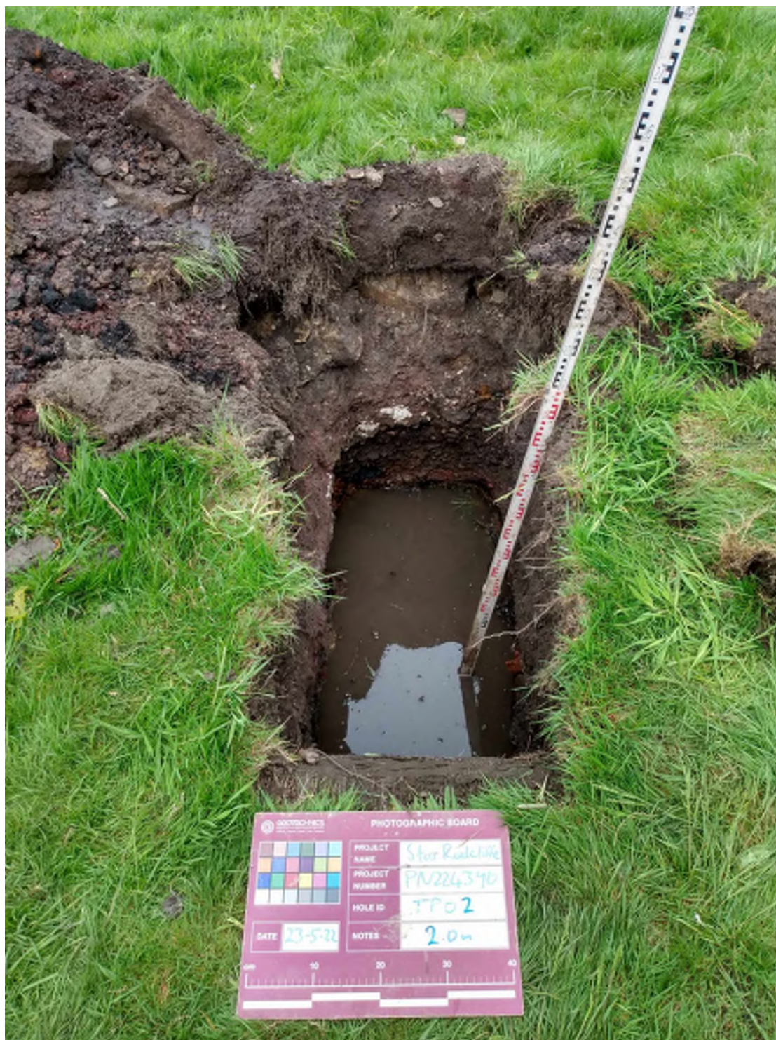
Machine-dug Trial Pit TP02 (I) during Soakaway Test
