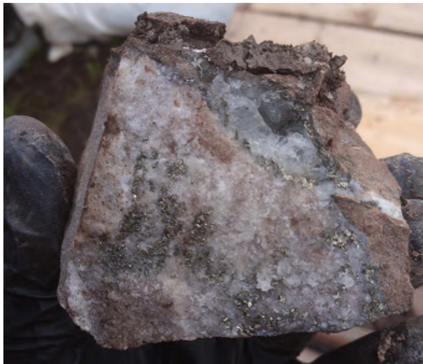
Borehole BH01 Box 1 of 9 18.55m-18.70m Quartz vein with pyrite
