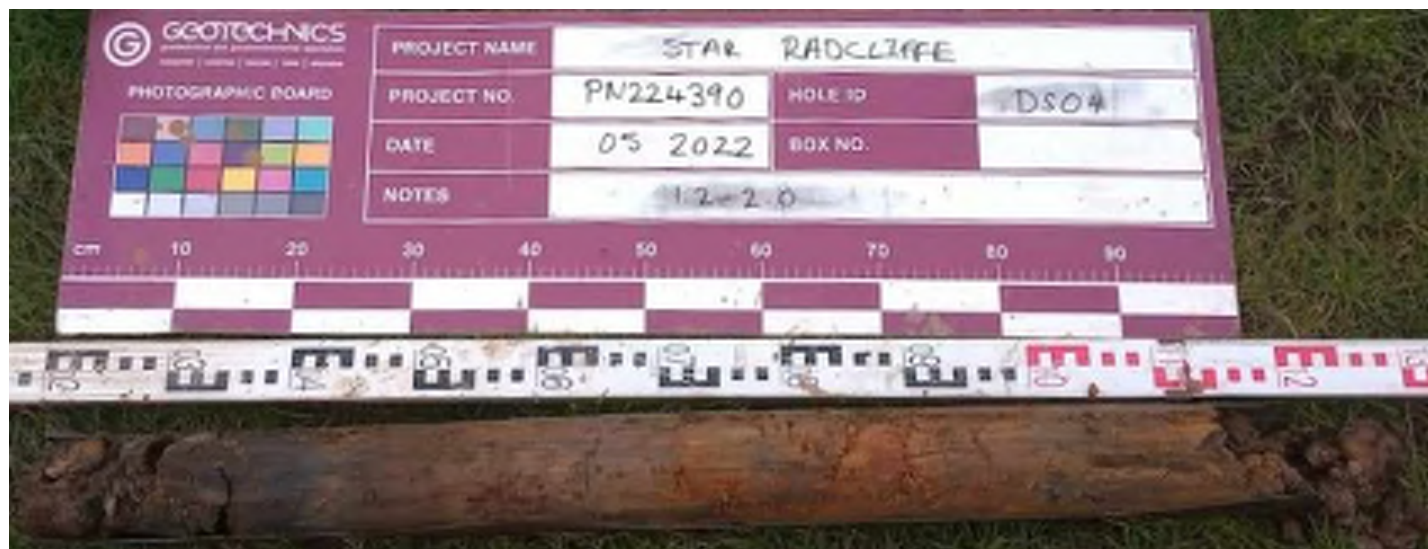
18) Dynamic Sample Borehole DS04 1.20m-2.00m
