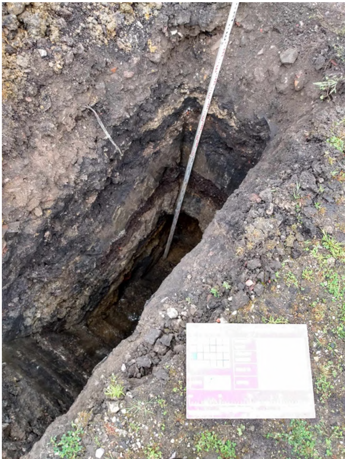
Machine-dug Trial Pit TP03 (2)
