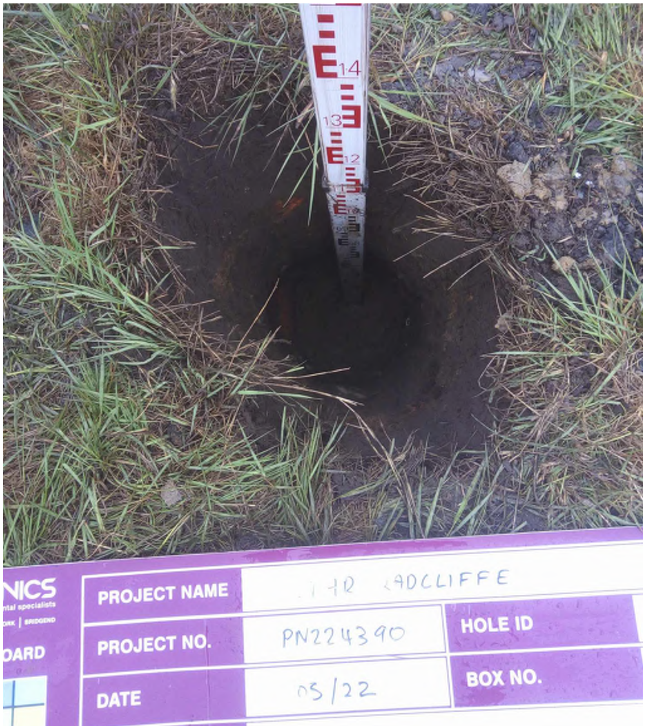
Hand-dug Trial Pit DCP08
