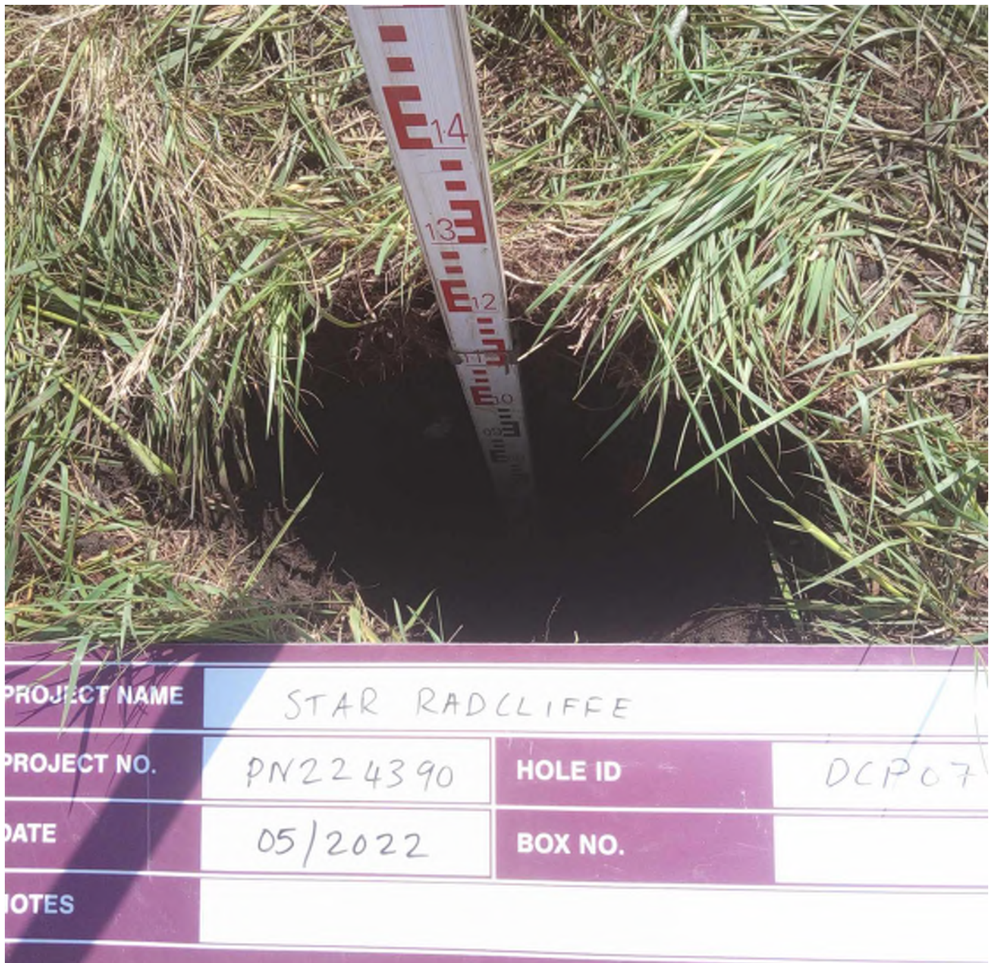
Hand-dug Trial Pit DCP07
