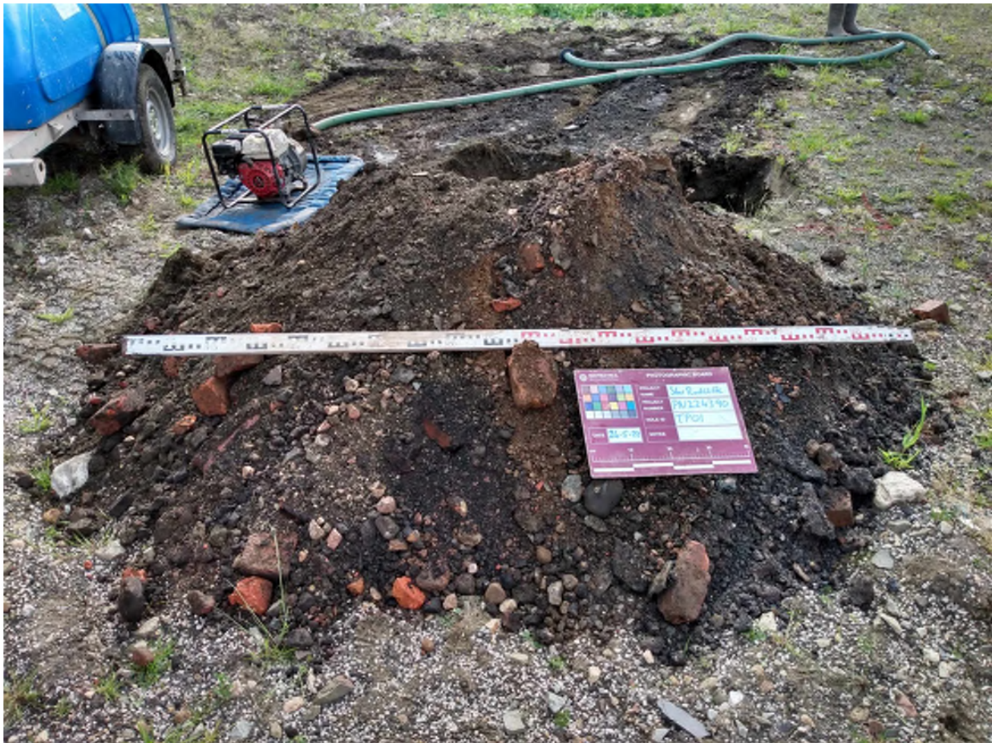
Machine-dug Trial Pit TP01 (3) Arisings
