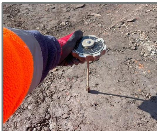
Hand shear vane testing
