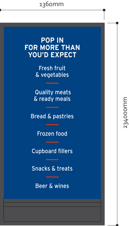
Sign B - 1:25 One PETG unit complete with display to match window frame. G/Cl - 145mm, depth 28mm.
