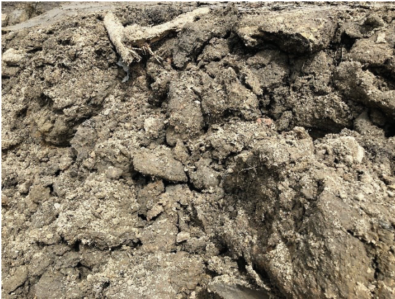
PLATE 9 SOFT/ORGANIC CLAY ENCOUNTERED DURING DRAINAGE EXCAVATIONS
