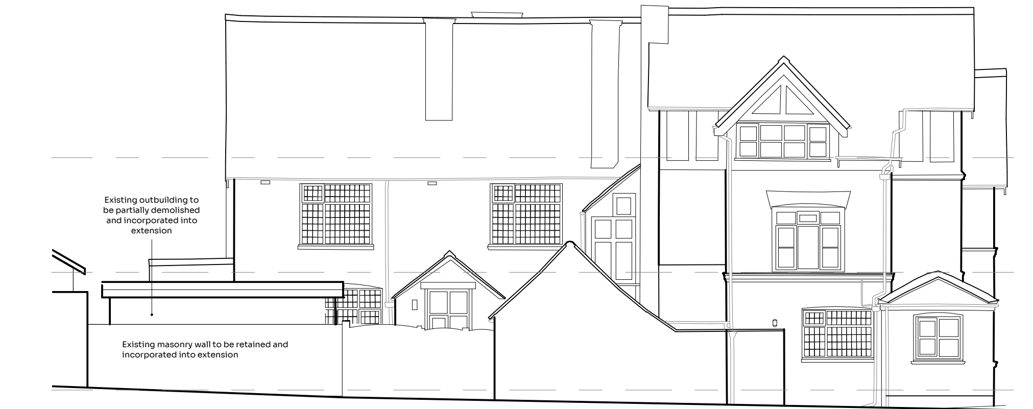
5 Elevation C - Existing
