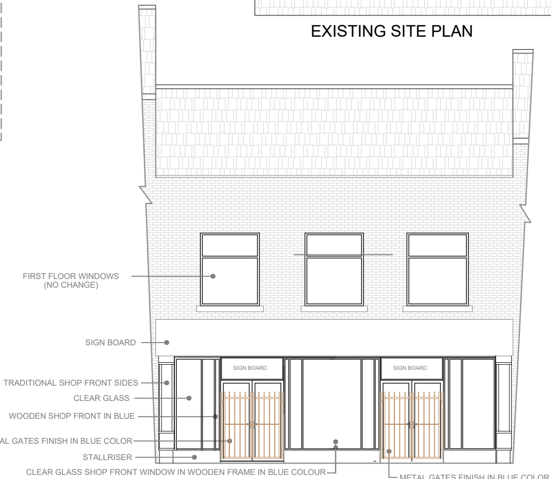
EXISTING FRONT ELEVATION
