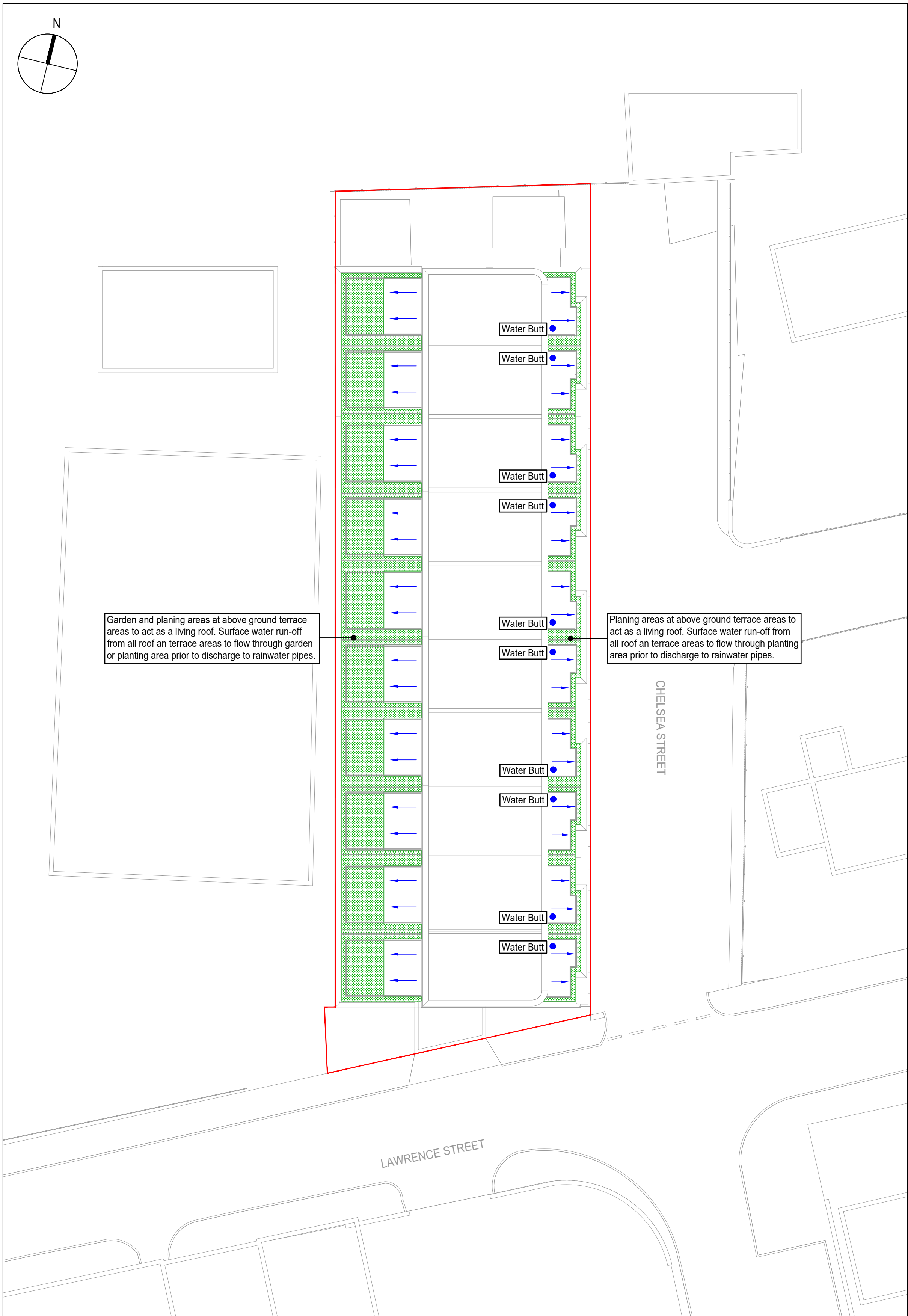
ABOVE GROUND SURFACE WATER MANAGEMENT LAYOUT
