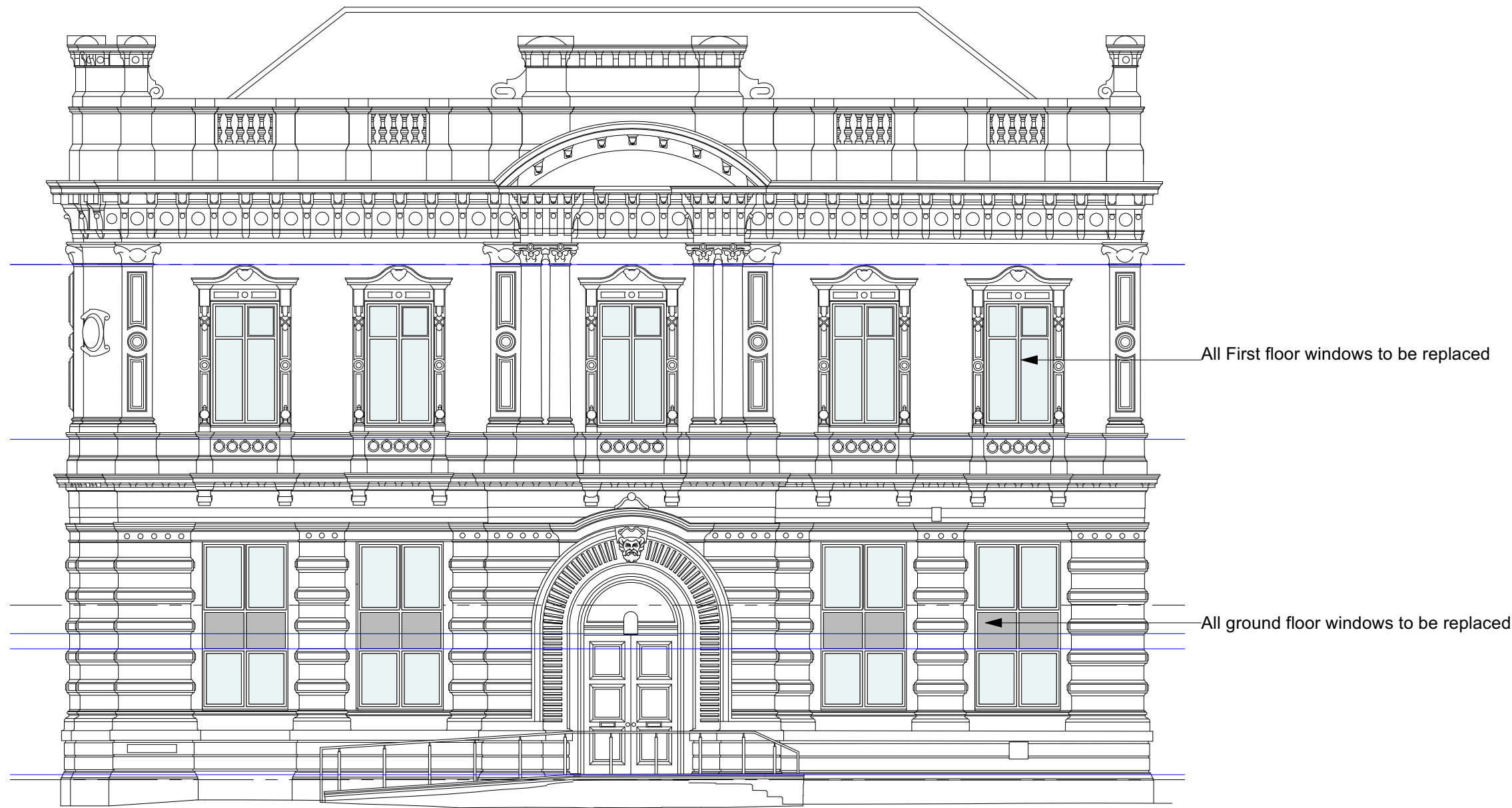
Front Elevation (Silver Street) As Proposed Scale 1:100
