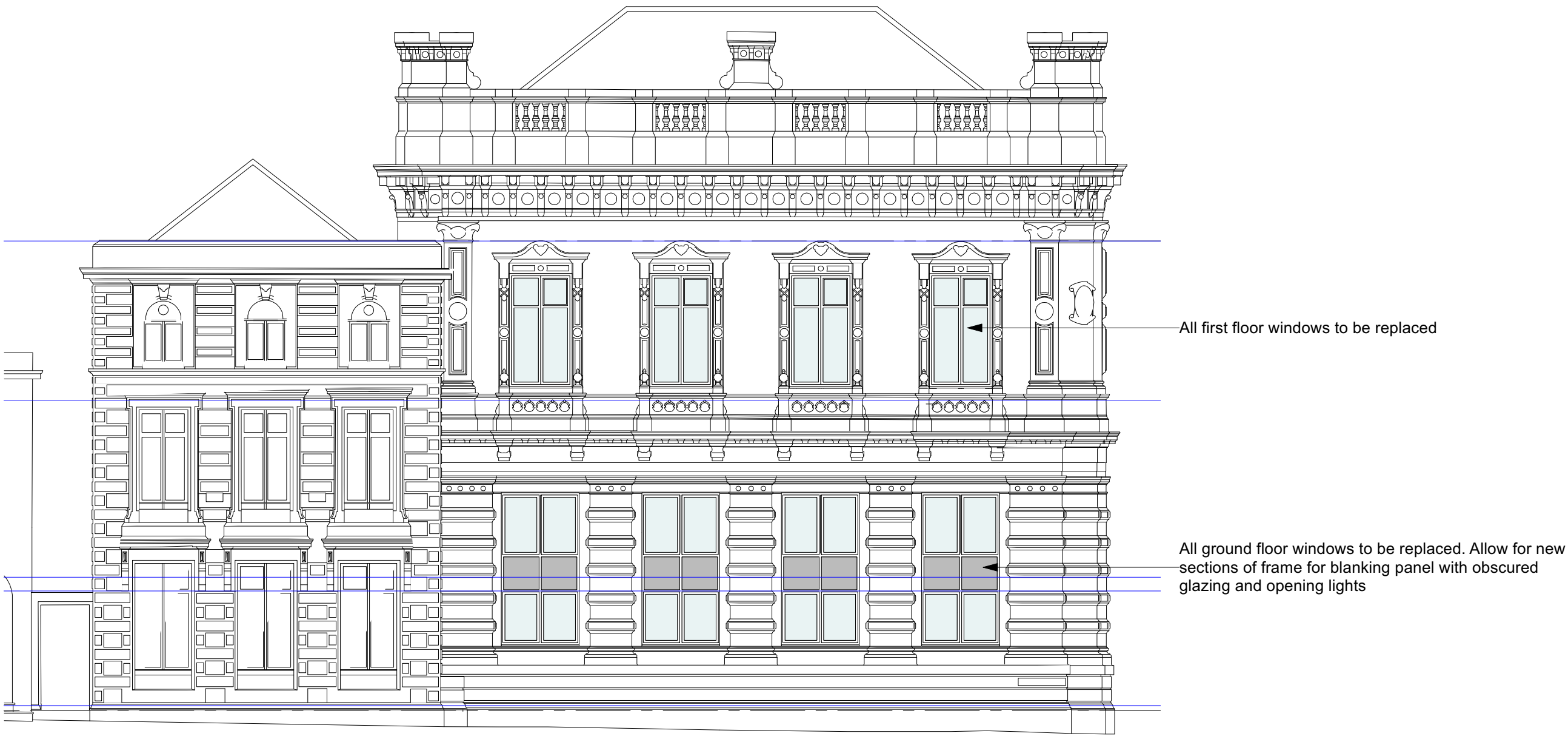
Side Elevation (Bank Street) As Proposed Scale 1:100
