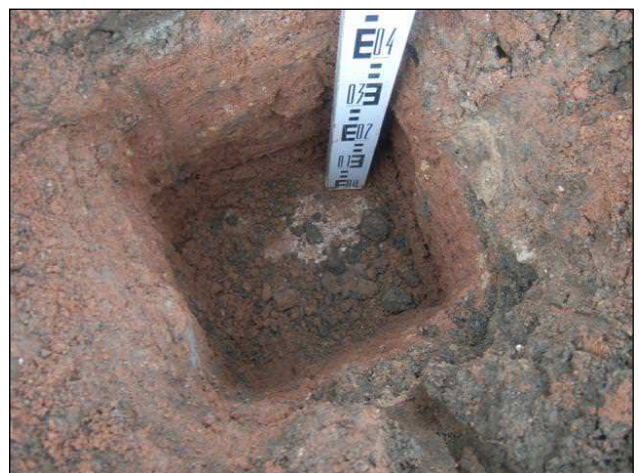
Photographs 15 and 16: Examples of validation photographs demonstrating inert cover depth and geotextile
