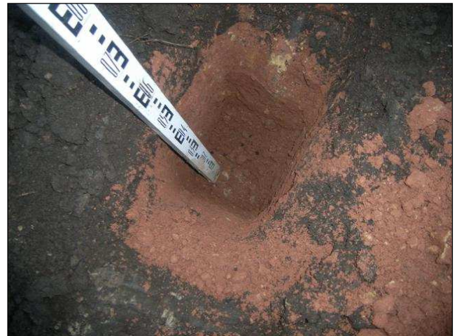
Photographs 13 and 14: Examples of validation photographs demonstrating validation hole location and soils forming inert cover
