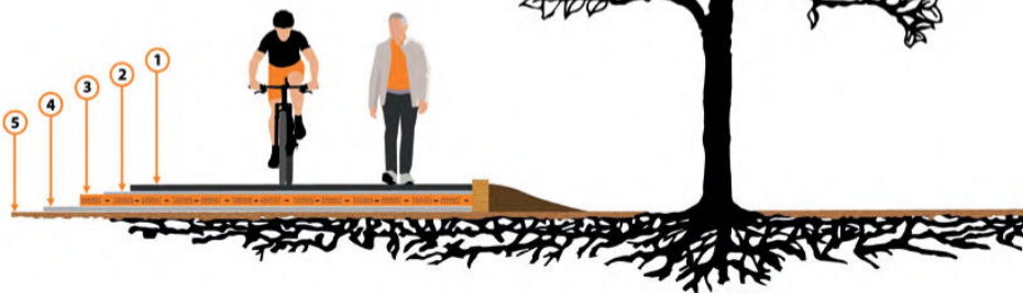
Figure 1: The basic approach to using cellular confinement systems for ground protection near trees [image courtesy of Core LP].
