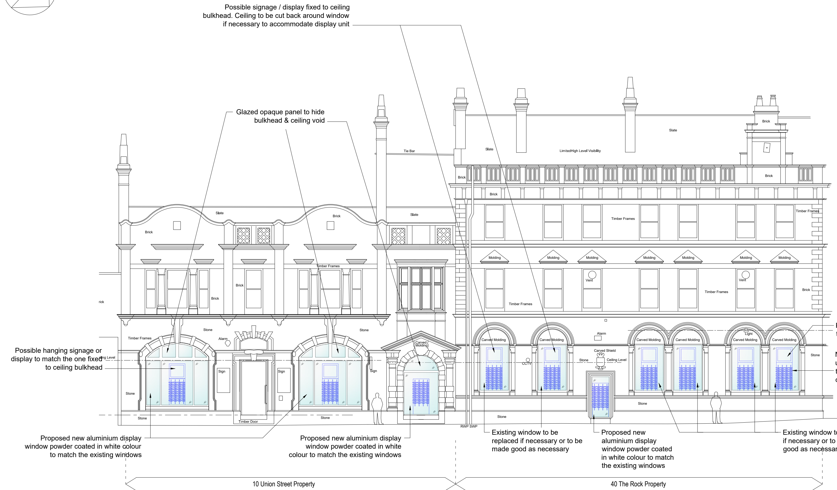
Proposed North East (Union Street) Elevation Scale 1:100
