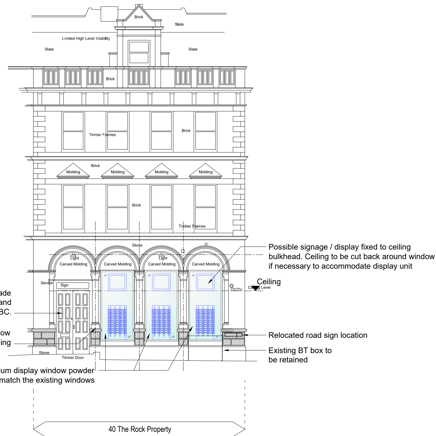
Proposed North West (The Rock) Elevation Scale 1:100
